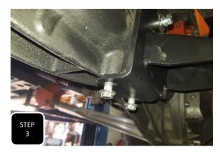
**Step 3** Loosely attach the new, center mounting bracket to the middle of the axle using the provided M10 bolts, washers, and aluminum spacers at the upper factory holes. Next, loosely install two of the factory bolts into the the lower mounting holes. **NOTE: THE SPACERS GO BETWEEN THE AXLE AND BRACKET.**
