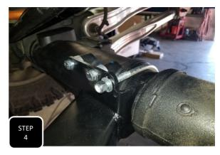
**Step 4** Slide the supplied 4.250" U-bolt around the axle housing and through the slotted holes in the center mounting bracket, then start the nuts/washers.
