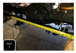
**Step 7** Loosely install the driver's side stabilizer mount on top of the tie rod using the provided 3/8" U-bolts, nuts, and washers. Measure from the stabilizer mounting hole on the center mounting bracket to the mounting hole the driver's bracket and adjust the bracket until you get a measurement of 20 inches. Next, make sure the mount is flat then torque the U-bolts to 30 ft/lbs.
