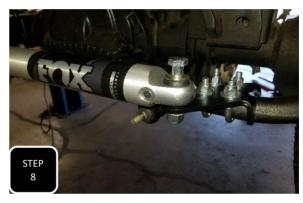
**Step 8** Loosely attach one of the steering stabilizers to the top of the center mounting plate using the supplied clevis/logo plate and 1/2" hardware. Next, loosely attach the other end of the stabilizer to the top of the driver's side bracket. **NOTE: THE STABILIZER CAN BE INSTALLED WITH THE BODY AT THE MIDDLE OR AT THE ENDS. THIS IS A**
