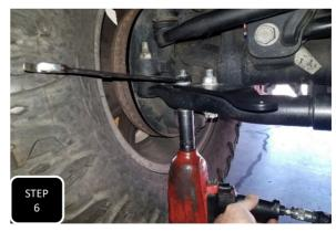
**Step 6** Attach the passenger side mounting plate to the tie rod using the factory bolts. Make sure the stabilizer mounting tab swoops downward and torque the bolts to 65 ft/lbs.
