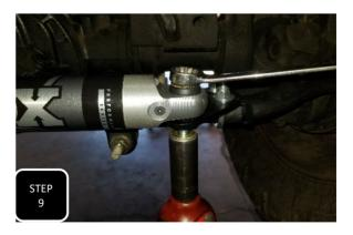
**Step 9** Loosely attach the other stabillizer to the passenger side mount and passenger side of the center clevis mount. Once all 4 mounting bolts have been loosely installed, torque the 1/2" bolts to 65 ft/lbs.
