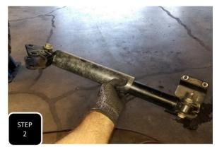
**Step 2** Unbolt and remove the 4 bolts attaching the factory steering stabilizer to the axle and then remove the factory stabilizer.
