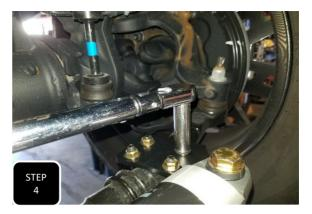
**Step 4** Loosely attach the driver side bracket using the provided 3/8" U-bolts/hardware, ensuring a level stance and confirming a measurement of 20 1/8" between the center bracket stabilizer hole and the stabilizer mounting hole of this bracket. Next, torque all of the 3/8" U-bolts to 30 ft/lbs.
