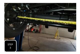
**Step 3** Locate the DS and PS mounting brackets. With the bent side facing downward, match up the brackets with the diagram above to determin which is which. Next, loosely install the pass side bracket using the provided 3/8" U-bolts/hardware. Before torquing, confirm a level stance of the bracket and a measurement of 20 1/8" between the stabilizer mounting hole on this bracket and the center mounting bracket.
