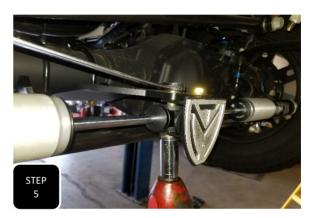
**Step 5** Loosely attach the steering stabilizers to the middle bracket using the provided clevis w/ MaxTrac logo and provided 1/2" bolt, nut, and washers. The stabilizer will mount to the bottom of the center bracket. **NOTE: IN SOME CASES, THAT STABILIZERS WILL NOT BE LEVEL. JUST LOOSEN THE MAIN U-BOLTS AND ROTATED THE BRACKET UNTIL THE STABILIZERS ARE LEVEL AND THEN RE-TORQUE THE U-BOLTS.**
