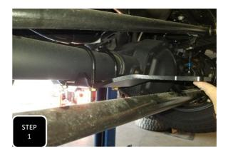
**Step 1** Locate the center mounting bracket and loosely attach it to the bottom of the middle of the axle using the supplied  $4.250" \times 1/2"$  Ubolts and hardware. Level the bracket and it will sit about 1" or so over the tie rod.
