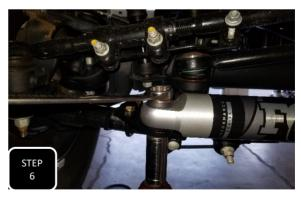
**Step 6** Attach the the other end of each stabilizer to the top of the outer mounts and torque all 4 mounting bolts to 60 ft/lbs.
