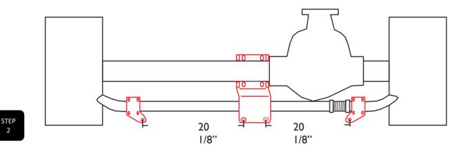
**Step 2** Push the bracket up against the side of the differential casting and then torque the U-bolts to 60 ft/lbs.
