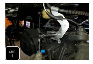
**Step 6** Unbolt the brake line brackets at the frame and at the axle to allow for slack when lowering the axle.
