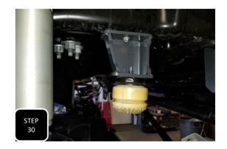
**Step 30** Attach the factory bump stop mounting cup to the bottom of the drop down bracket using the provided M8 bolt, nut, and washers. Once tight, then pop the factory bump stop back in.
