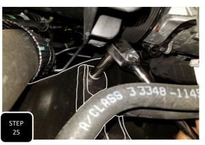
**Step 25** Remove the two mounting bolts that attach the factory steering stabilizer bracket to the passenger side frame and separate.
