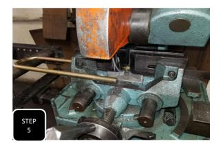
**Step 5** Depending on what leaf pack is in your truck, the U-bolts included in this kit may need to be cut down. If this is the case, install them, measure how much you want to cut off, and then do so for the cleanest install possible.
