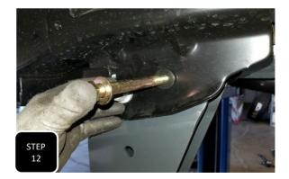
**Step 12** Install the radius arm drop down bracket into the factory radius arm bracket on the frame and loosely attach it using the factory bolt at the big hole and the provided small machined washers along with the provided 9/16" bolt at the small hole. **NOTE: THE SMALL MACHINED WASHERS GET INSTALLED FROM THE OUTSIDE OF THE BRACKET FACING INWARD.**
