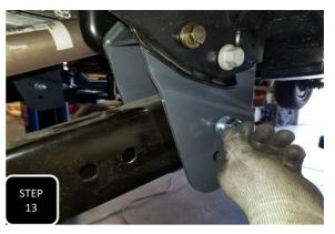
**Step 13** Swing the radius arm up and attach it to the new bracket using the provided M18 bolt. For a 4" lift attach the arm to the upper of the two holes and for a 6" lift attach it to the lower of the two holes.
