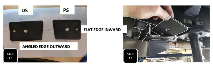
**Step 17** Locate the flat plate labeled DS and slide it into the cross member above the back of the 4 link bracket. Line up the holes and loosely attach the plate and bracket together using the provided 3/8" and 5/16" socket head allen bolts. **NOTE: THE DRIVER'S SIDE IS THE LONGER PLATE**
