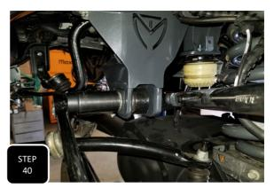
**Step 40** When attaching the trac bar to the drop down bracket, you will need to use the provided off-set plates. The hole will need to be off-set to the driver's side for the 4" lift or towards the passenger side for the 6" lift. Use the factory M18 bolt and nut and only loosely attach for now. **NOTE: THE TRAC BAR WILL GET FULLY TIGHTENED WHEN THE TRUCK IS ON THE GROUND AT RIDE HEIGHT.**
