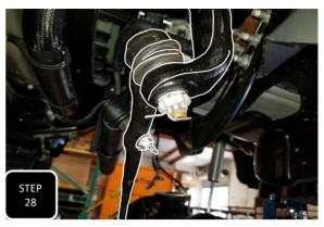
**Step 28** Attach the drag link to the pitman arm, from the top down, using the factory nut and tighten. Next, install the castle sleeve and the factory cotter pin.
