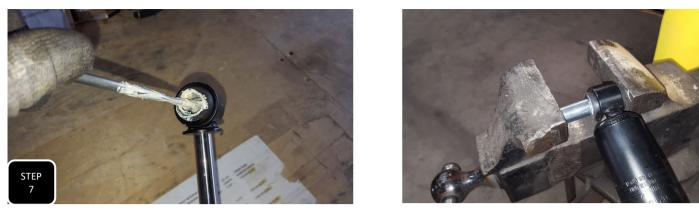
**Step 7** If installing Max Trac shocks, you will need to grease the bushings and use a bench vise to press in the shock sleeves.
