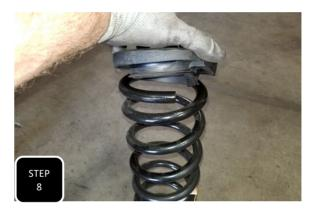
Step 8 Lower down the axle and remove the coil. Separate the rubber isolator and save for use on the new coils.
