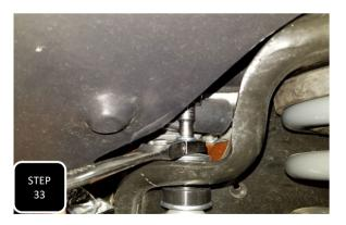
Step 33 Tighten up both ends of both front shocks.
