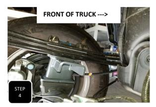
**Step 4** Working on one side at a time, remove the U-bolts and lower the axle down enough to remove the factory lift block and install the new, taller lift block. The block will need to be installed with the shorter side facing the front of the truck and with the bump stop stiker plate facing inward.
