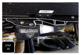
**Step 16** Loosely install the 4 link bracket using the provided M18 bolt at the large hole and the 9/16 x 5" bolt along with the small machined washers at the small hole. **NOTE: THE MACHINED WASHERS WILL SLIDE IN THE FRAME HOLE ON THE OUTSIDE OF THE FACTORY BRACKET.**
