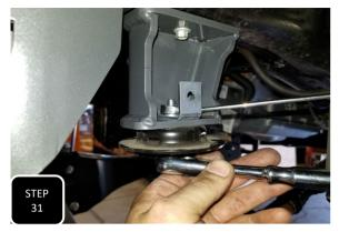
**Step 31** On the driver's side you will need to attach the 90 degree ABS line mounting bracket to the bolt used to attach the bump stop mounting cup.
