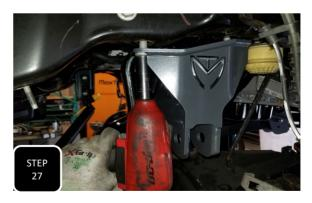
**Step 27** Locate the new trac bar bracket and attach it using the the factory nuts/3 bolt plate at the cross member and the factory 2 bolts under the frame then tighten.
