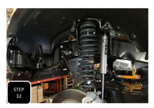
**Step 32** Move your adjustable jack under the driver's side of the axle and apply pressure so that you can remove the lower shock bolt and then lower the axle down. Next, Install the new lift coil with the factory rubber isolator on top, jack the axle back up and re-attach the shock. Repeat this step on the other side.
