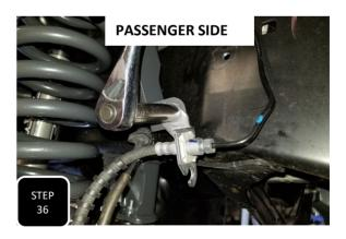
**Step 36** The passenger side ABS/ brake line bracket will mount the same as the driver's side and also require the unraveling of the factory hard brake line to line up with the new bracket.
