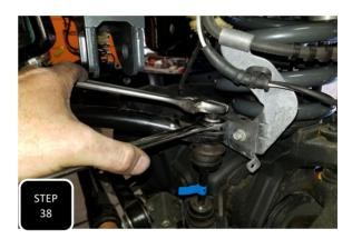
**Step 38** Attach the sway bar to the drop down brackets using the provided M10 bolts, nuts, and washers then tighten. Next, re-attach the ends to the end links on the axle using the factory nuts and tighten.
