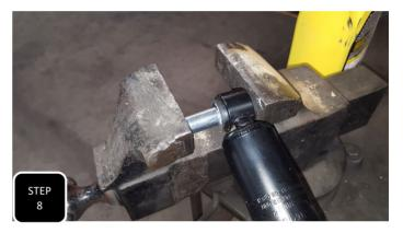
**Step 8** If installing Max Trac shocks, you will need to grease the bushings and use a bench vise to press in the shock sleeves.
