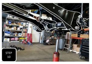
**Step 10** Once both sides have the coils removed and are supported by the new shocks, move the adjustable jack to the middle of the axle and apply pressure.
