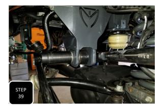
**Step 39** When attaching the trac bar to the drop down bracket, you will need to use the provided off-set plates. The hole will need to be off-set to the driver's side for the 4" lift or towards the passenger side for the 8" lift. Use the factory M18 bolt and nut and only loosely attach for now. **NOTE: THE TRAC BAR WILL GET FULLY TIGHTENED WHEN THE TRUCK IS ON THE GROUND AT RIDE HEIGHT.**
