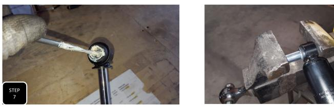
**Step 7** If installing Max Trac shocks, you will need to grease the bushings and use a bench vise to press in the shock sleeves.
