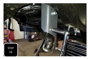
**Step 26** Using the provided M10 bolts and washers, attach the new steering stabilizer drop down bracket to the inside of the passenger side frame with the welded shim touching the frame and tighten. Next, attach the factory bracket to the lower half of the drop down bracket using the other provided M10 bolts, nuts, and washers. **NOTE: THE FACTORY BRACKET WILL MOUNT INSIDE OF THE PROVIDED BRACKET.**
