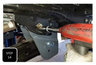
**Step 14** Repeat steps 11-13 on the driver's side and then tighten the bolts attaching the bracket to the frame, the big bolt gets torqued to 200 ft/lbs and the smaller one to 130 ft/lbs. The radius arm bolts will not get tightened until the truck is on the ground at ride height.
