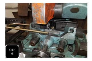
**Step 6** Depending on what leaf pack is in your truck, the U-bolts included in this kit may need to be cut down. If this is the case, install them, measure how much you want to cut off, and then do so for the cleanest install possible.
