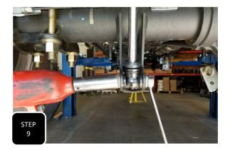
**Step 9** Install your new longer shocks using the factory hardware and tighten. **NOTE: MAX TRAC SHOCKS HAVE TO BE MOUNTED WITH THE BODY OF THE SHOCK AT THE AXLE AND THE SHAFT OF THE SHOCK AT THE FRAME. FOX SHOCKS WILL BE MOUNTED THE OPPOSITE OF THIS.**
