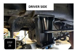
**Step 29** Pop the factory bump stop out of its mounting cup then unbolt the cup and using the same bolt, attach the new bump stop drop down bracket to the same mounting hole. The angled side of the bracket will face the rear of the truck, the shorter of the two surfaces downward, and the open end outward.
