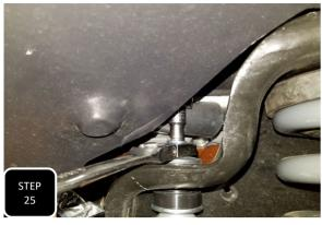
**Step 25** Tighten up both ends of both front shocks.
