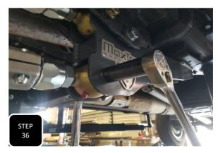
**Step 36** If you installed the MaxTrac 4 links, torque the axle side bolts to 200 ft/lbs and the frame side bolts to 100 ft/lbs. If you purchased the radius arm bracket kit then torque all 6 radius arm bolts to 200 ft/lbs.
