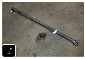
**Step 10** Unbolt the trac bar from the frame and remove the trac bar. **NOTE: SAVE THE MOUNTING BOLT FOR THE INSTALL OF THE NEW TRAC BAR.**
