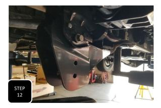
**Step 12** Install the radius arm drop down bracket into the factory radius arm bracket on the frame and loosely attach it using the factory bolt at the big hole and the provided  $3/8-16 \times 41/2$ " bolt at the small hole.
