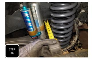
**Step 36** Install the wheels and tires then lower the truck back down to ride height. Drive the truck backwards about 10 feet and then forward about 10 feet to settle the suspension. Next, take a measurement from the inside of the front tire to the frame on both sides (in a consistant spot) and then compare your measurements.
