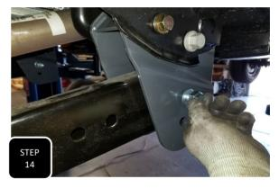
Step 14 Swing the radius arm up and attach it to the new bracket using the provided M18 bolt, nut, & washers.
