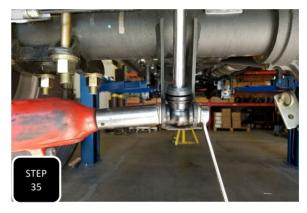
**Step 35** Install your new longer shocks using the factory hardware and tighten. **NOTE: MAX TRAC SHOCKS HAVE TO BE MOUNTED WITH THE BODY OF THE SHOCK AT THE AXLE AND THE SHAFT OF THE SHOCK AT THE FRAME. FOX SHOCKS WILL BE MOUNTED THE OPPOSITE OF THIS.**
