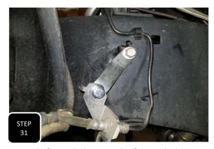
**Step 31** Attach the passenger side, shorter bracket to the passenger side frame hole using the factory bolt. Next, gently unravel the factory hardline until the factory bracket reaches the new mounting hole on the provided bracket and attach the two using the provided M8-1.25 x 20mm bolt, nut, and washers.
