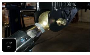
**Step 20** Locate the other arm that matches the one you just installed, adjust it to an eye-eye length of 32 1/2" and grease the rod end. Next, loosely install it into the bottom hole of the 4 link frame bracket using the provided 9/16" bolt, washers, and nut. **NOTE: THE ROD ENDS ARE NOT PRE-GREASED AND REQUIRE GREASE FOR PROPER FUNCTION.**
