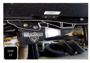
**Step 17** Loosely install the 4 link bracket using the provided M18 bolt at the large hole and the 3/8-16 x 4 1/2" bolt at the small hole.
