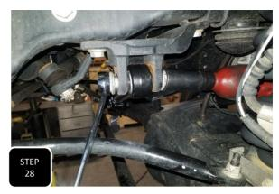
**Step 28** Loosely attach the new, adjustable trac bar to the frame using the factory bolt and only snug up the bolt. **NOTE: THIS BOLT WILL NOT GET FULLY TIGHTENED UNTIL THE TRUCK IS BACK ON THE GROUND AT RIDE HEIGHT.**
