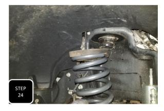
**Step 24** Move your adjustable jack under the driver's side of the axle and apply pressure so that you can remove the lower shock bolt and then lower the axle down. Next, Install the new lift coil with the factory rubber isolator on top, jack the axle back up and re-attach the shock. **Repeat this step on the other side.**
