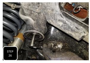
**Step 26** Pry the factory bump stop out of its mounting cup on the frame and then remove the single mounting bolt and mounting cup.
