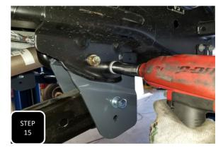
**Step 15** Repeat steps 11-14 on the passenger's side and then tighten the bolts attaching the bracket to the frame, the M18 bolt gets torqued to 200 ft/lbs, the 3/8" to 45 ft/lbs and the M12 socket head bolt to 50 ft/lbs. The radius arm bolts will not get tightened until the truck is on the ground at ride height.
