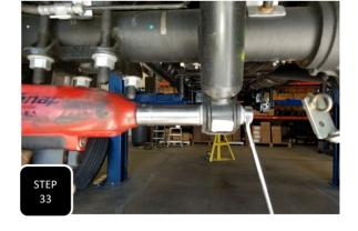
**Step 33** Unbolt both rear shocks at both ends and remove.
