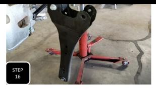
**Step 16** Loosen all 3 radius arm mounting bolts, 2 at the axle and 1 at the frame and then remove the radius arm. **NOTE: WORK ON ONE SIDE AT A TIME.**
