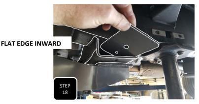
**Step 18** Locate the flat plate labeled DS and slide it into the cross member above the back of the 4 link bracket. Line up the holes and loosely attach the plate and bracket together using the provided M12" socket head allen bolt. Once all of the bolts have been installed, torque the large, M18 bolt to 200 ft/lbs and both the 3/8" and M12 socket head allen bolt to 50 ft/lbs. **NOTE: THE DRIVER'S SIDE IS THE LONGER PLATE**
