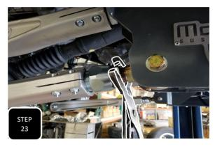
Step 23 Tighten down all 4 of the M8 pinch bolts and then cinch down the two jam nuts on the rod ends.
