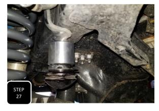
**Step 27** Locate the provided bump stop extensions and install them between the bump stop mounting cup and the frame using the supplied M8-1.25 x 75mm bolts and torque to 18 ft/lbs. Next, spray some WD-40 on the bump stop and pop it back into the mounting cup.
