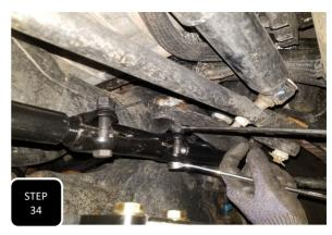
**Step 34** Loosen up the adjustment clamps on the trac bar and adjust the trac bar accordingly until your measurements match each other. Next, tighten down both clamps on the collar.
