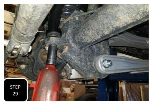
**Step 29** Loosen the adjustment collar of the trac bar and adjust the length until the rod end drops into the mounting hole on the axle. Next, torque the nut to 200 ft/lbs. **NOTE: FINAL ADJUSTMENTS WILL BE MADE WHEN THE TRUCK IS BACK ON THE GROUND AT RIDE HEIGHT.**
