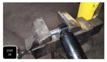
**Step 34** If installing Max Trac or Vulcan series shocks, you will need to grease the bushings and use a bench vise to press in the shock sleeves.
