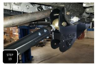
**Step 19** Locate 1 of the 4 arms. There should be 2 DS where the "MT" logo is facing up and the pinch bolts are facing outward. The PS arms are the opposite. Adjust the arm to a length of 32" from eye-eye with the grease fitting facing downward. Next, grease the rod end and loosely install it into the upper part of the 4 link frame bracket where you previously loosely installed the provided 9/16" bolt. **NOTE: THE ROD ENDS ARE NOT PRE-GREASED AND REQUIRE GREASE FOR PROPER FUNCTION.**
