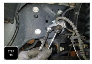
**Step 30** Locate the provided brake line brackets. The longer one is for the driver's side. Attach the side with the bent tab to the frame using the factory bolt. Next, gently unravel the factory hard brake line until it reaches the new mounting hole. You will want to separate the ABS line and re-route it around the factory brake line bracket, then
