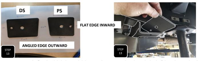
**Step 13** Locate the flat plate labeled DS and slide it into the cross member above the back of the radius arm bracket. Line up the hole and loosely attach the plate and bracket together using the provided M12-1.5 X 40 socket head allen bolt. **NOTE: THE DRIVER'S SIDE IS THE LONGER OF THE TWO PLATES.**
