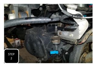
**Step 2** Unbolt the sway bar from the end link on both sides and separate.
