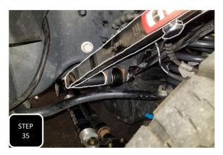
**Step 35** Torque the trac bar bolt at the frame to 406 ft/lbs.
