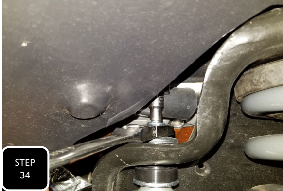
Step 34 Tighten up both ends of both front shocks.
