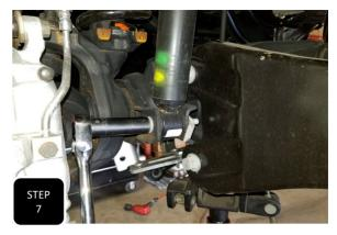
**Step 7** Move the adjustable jack to the driver's side and apply pressure to the axle. Next, unbolt the driver's side shock at both ends and remove.
