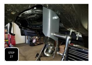
**Step 27** Using the provided M10 bolts and washers, attach the new steering stabilizer drop down bracket to the inside of the passenger side frame with the welded shim touching the frame and tighten. Next, attach the factory bracket to the lower half of the drop down bracket using the other provided M10 bolts, nuts, and washers. **NOTE: THE FACTORY BRACKET WILL MOUNT INSIDE OF THE PROVIDED BRACKET.**
