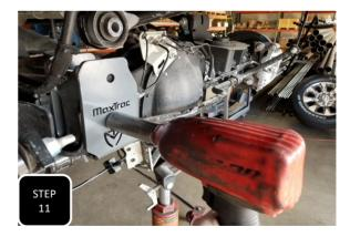
**Step 11** Tighten down the 3/8" bolt at the bottom of the trac bar bracket. The easiest way to hold the head of the bolt tight is to wedge a flat head screw driver down against the head. Next, tighten down the bolt in the original trac bar mounting hole.
