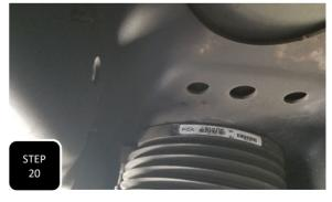
**Step 20** Install the wheels/tires and lower the vehicle down to the ground, but with the lift still holding the weight of the vehicle. First, ensure that the top of the air bag is properly aligned in the guide hole of the frame and then, second, turn the ignition on and allow the air bags to fill up before lowering the lift completely to the ground.
