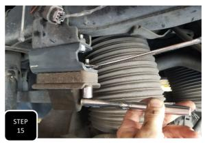
**Step 15** Unbolt the factory bump stops along with the 1" spacers. Next, install the bump stop extension brackets with the notched edge facing the back of the truck and the open end facing inward using the provided bolts and washers. Next, attach the factory bump stops along with the factory 1" spacer to the new bracket using the factory bolts and provided nuts/washers. Once everything is loosely attached, tighten it up.
