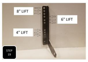
**Step 19** There are 9 mounting holes on the new sensor bracket. The 3 lowest holes are for a 1.5" rear lift, the 3 middle holes are for a 3.5" rear lift, and the 3 upper holes are for a 5.5" rear lift. Install the factory mounting ball into the desired hole using the provided M6 nut and washer then attach the sensor rod to it. **NOTE: THE MIDDLE HOLE OF EACH SET OF HOLES IS THE STARTING HOLE AND THE ABOVE OR BELOW HOLES WILL LIFT OR LOWER THE REAR OF THE TRUCK BY ABOUT 1/2".**
