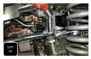
**Step 44** Attach the sway bar to the drop down brackets and to the axle using the provided hardware at the brackets and the factory nuts at the axle then tighten them all down. **NOTE: IT WILL EASE THE INSTALL TO FIRST LOOSELY ATTACH THE SWAY BAR TO THE END LINKS AND THEN TO THE BRACKETS ON THE FRAME.**
