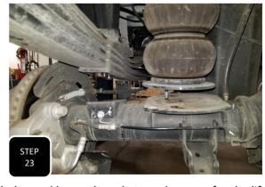
**Step 23** One side at a time, loosen both U-bolts, remove the U-bolts, and lower the axle to make room for the lift block. **NOTE: IT WILL HELP THE ALIGNMENT OF THE LIFT BLOCK TO SLIGHLY LOOSEN THE U-BOLTS ON THE OTHER SIDE.**
