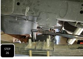
**Step 26** Jack up the rear axle to seat both the block and spacer, install the U-bolts, and torque them to 100 ft/lbs. Next, tight both new bolts from the spacer to the axle as well as both studs attaching the spacer to the air bag.
