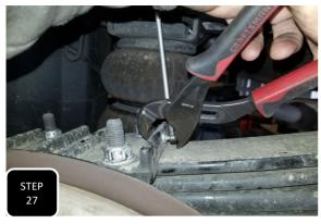
**Step 27** Re-attach the sensor rod to the spring plate using a set of channel locks to help pop the sock back onto the mounting ball then move to the other side and repeat steps 15-21 on the other side.
