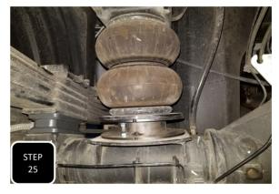
Step 25 Before jacking up the axle and seating the block/air bag spacer, insert the new mounting bolts into the bottom plate from the top down and get the nut started on factory stud. NOTE: WITH THE 1.5" REAR LIFT, THERE WILL NOT BE ROOM TO INSERT THE NEW BOLT WHEN THE STUD IS COMPLETELY INSERTED.
