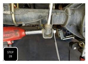
**Step 28** Install the new shocks and tighten. Max Trac shocks need to be installed with the shaft of the shock at the frame and the body at the axle. Fox shocks get installed opposite of that.
