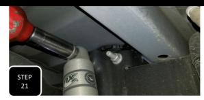
**Step 21** Jack up the rear of the truck and support under the frame with jack stands. Apply pressure to the rear diff with an adjustable jack and remove both rear shocks.
