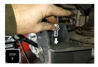
**Step 8** Slide the new trac bar bracket over the factory trac bar bracket on the axle and loosely install the factory bolt through the original trac bar mounting hole with the provided crush tube in the middle. Next, install one of the provided 3/8" bolts and washers through the inside, bottom of the bracket. **NOTE: DO NOT FULLY TIGHTEN EITHER OF THESE BOLTS AT THIS TIME.**
