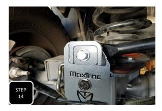
**Step 14** The plates with the off-center hole will get installed with the bolt towards the driver's side for the 4" and 6" lift. Its only off-set to the pass side for the 8" lift. **NOTE: DO NOT TIGHTEN UNTIL THE TRUCK IS ON THE GROUND AT RIDE HEIGHT.**
