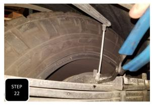
**Step 22** Unbolt both air bag bolts on the side you are working on and then disconnect the sensor rod from the spring plate by popping the socket off of the mounting ball.
