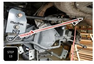
**Step 13** Use a rachet strap to pull the axle over and align the trac bar with the hole in the new bracket then loosely attach with the provided square plates and M14 bolt.
