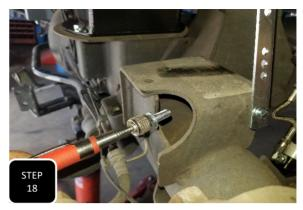
**Step 18** Unbolt the sensor rod ball from the mount on the axle and install the provided sensor brackets using the M6 bolt/washer at the original hole and the provided M8 bolt, nut & washer at the blank hole around the corner from the original bolt. **NOTE: USING A MAGNET WILL EASE THE PROCESS OF INSTALLING THE BOLT IN THE BLOCK ON THE AXLE.**
