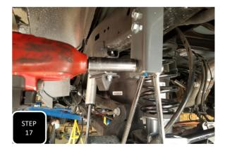
**Step 17** Attach the sway bar drop down bracket to the factory sway bar bracket using the provided 7/16" hardware and tighten. Next, attach the sway bar end link to the new bracket using the factory hardware and tighten. Repeat on other side.
