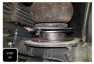
**Step 24** Install the lift block and the air bag spacer. The airbag spacer is off-set and when installed properly, the upper plate should off-set towards the rear of the truck with the ovalized holes facing the rear of the truck.
