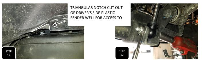
Step 12 Install the new shocks and tighten down both ends. NOTE: DO NOT OVER TIGHTEN THE TOP BUSHING OF THE SHOCK OR THE BUSHING WILL NOT BE ABLE TO FLEX AND COULD DAMAGE TO THE SHOCK.
