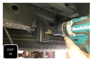
**Step 16** Loosely attach the sway bar drop down bracket to the factory bracket on the frame and mark the upper hole for drilling. Remove the bracket and drill a 7/16" hole at your mark. **NOTE: USING A STEP BIT WILL SPEED UP THE DRILLING.**
