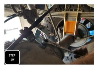
**Step 19** Unbolt the brake line bracket and E-brake loom clamp on top of the differencial and attach the provided brake line bracket using the factory stud and nut.
