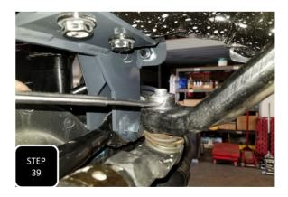
Step 39 Attach the tie rod to the pitman arm from the bottom up and tighten.
