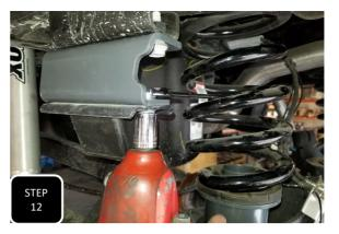
**Step 12** Unbolt the factory bump stops and install the bump stop extension brackets with the notched edge facing the back of the truck and the open end facing inward. Next, attach the factory bump stops to the new bracket using the provided M10 hardware and tighten.
