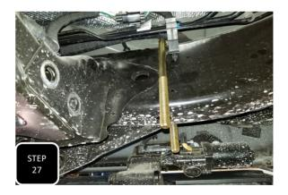
**Step 27** Working at the front of the cross member, pry the plastic fuel line guide bracket away from the frame and install the provided U-bolt over the frame from the top down with the shorter leg of the U-bolt on the inside of the frame.
