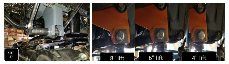
**Step 37** Slide the trac bar up into the new drop down bracket and loosely attach it using the provided M18 hardware and square plates with off-set hole. Install the plate so that the bolt is off-set to the passenger side of the truck. **NOTE: DO NOT FULLY TIGHTEN THIS BOLT UNTIL THE TRUCK IS ON THE GROUND AT RIDE HEIGHT.**
