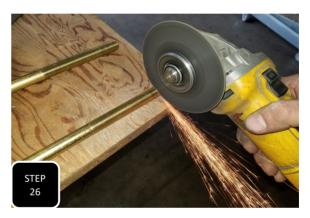
**Step 26** Locate the provided 9" long, square U-bolts for the 4link brackets, mark a cut line 1/2" down the threads of "only" one side, then cut that leg of the U-bolt on that line so that it is 1/2" shorter.
