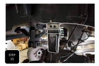
**Step 15** Attach the new bump stop bracket to the frame using the provided 1/2" bolts and then attach the factory bump stop cup to the new bracket using the provided 3/8" bolts, nuts, & washers. Next, spray some WD-40 onto the provided bump stop and pop it into the factory cup. **NOTE: JACKING UP THE AXLE AND USING IT TO PRESS THE BUMP STOP IN THE CUP WILL MAKE THIS MUCH EASIER.**
