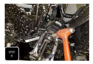
**Step 9** Remove the nut attaching the pitman arm to the steering box and then using a pitman arm puller or suitable 3 jaw puller, apply tension to the pitman arm and hit the side of the pitman arm with a hammer. After a few hits, tighten down the puller again and then repeat with the hammer until the arm separates.
