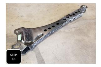
**Step 18** Starting with the passenger side, remove the previously loosened radius arm bolts and then remove the radius arm. **NOTE: ONLY REMOVE ONE RADIUS ARM AT A TIME.**
