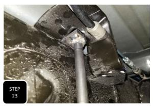
**Step 23** Loosely install the radius arm drop down bracket into the original mount using the factory bolt and then loosely attach the provided 1/2-13 x 9" bolts, washers, and lock washers to the nut plate on top of the frame. Push the bracket up tight to the frame and torque the factory bolt to factory specs and the 1/2" bolts to 90 ft/lbs.
