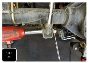
**Step 21** Install the new shocks and tighten. Max Trac shocks need to be installed with the shaft of the shock at the frame and the body at the axle. Fox shocks get installed opposite of that.
