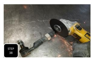
**Step 38** Loosen the clamp on the tie rod and remove the rod end. Using a suitable cutting device, cut off the half circle end piece after the threads and then thread the rod end back into the sleeve, leaving the rod end pointing upward now instead of downward like it was from the factory.
