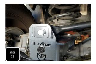
**Step 11** Use a rachet strap to pull the axle over and align the trac bar with the slotted hole and two square plates with the off-center hole. Off-set the bolt towards the passenger side of the truck for 8" lift. **NOTE: DO NOT TIGHTEN UNTIL THE TRUCK IS ON THE GROUND AT RIDE HEIGHT.**
