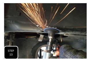
Step 13 Once removed, clean up all sharp edges with a sander and then spray paint the frame to prevent rust.
