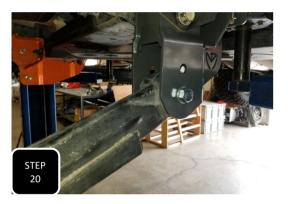
Install the radius arm into the: Upper hole for the 4" lift Lower hole for the 6" and 8" lift.
