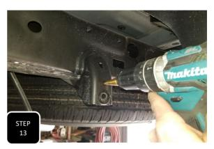
**Step 13** Loosely attach the sway bar drop down bracket to the factory bracket on the frame and mark the upper hole for drilling. Remove the bracket and drill a 7/16" hole on your mark. **NOTE: USING A STEP BIT WILL SPEED UP THE DRILLING.**
