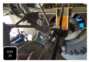
**Step 20** Attach the brake line bracket and E-brake cable guide to the top holes of the provided bracket using the provided 1/4" bolts, nuts, & washers.
