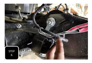
**Step 6** Unbolt the brake line bracket on both axles and unclip the wiring harness for the 4wd module.
