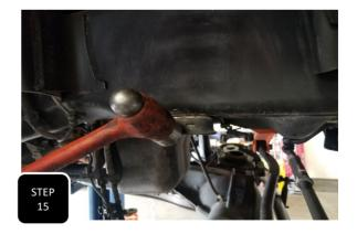
**Step 15** Using a suitable cuting device, cut the welds of the factory bump stop cup and then hit it with a hammer to break it loose. **NOTE: TRY NOT TO DAMAGE OR DISTORT THE CUP AS IT NEEDS TO BE RE-USED.**
