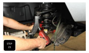
**Step 23** Install the steering knuckle assembly onto the the appropriate side that you are working on with the steering arm of the knuckle facing the front of the truck. Use the factory nuts at the upper and lower ball joints and tighten to factory specs. **NOTE: SLIDE THE AXLE INTO THE HUB BEFORE CONNECTING THE BALL JOINTS.**
