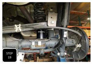
**Step 19** Loosely attach the trac bar to the new drop down bracket using the factory bolt and nut. **NOTE: DO NOT FULLY TIGHTEN THIS BOLT UNTIL THE TRUCK IS BACK ON THE GROUND AT RIDE HEIGHT.**
