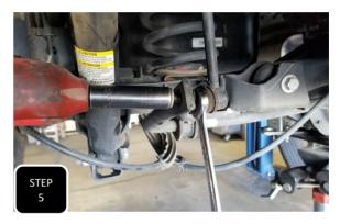
**Step 5** Unbolt both sway bar end links at both ends and remove.
