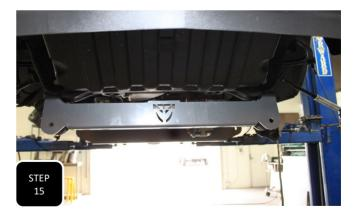
**Step 15** Loosely install the front subframe with the logo facing forward, using the factory hardware.
