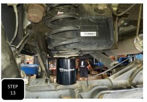
**Step 13** Locate the coil spacers and loosely install them along with the factory coils and isolators. Once both are in place, jack up the axle to apply pressure to the coils and assure that they are properly seated.
