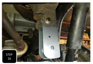
**Step 16** Loosely install the provided trac bar bracket onto the factory trac bar bracket on the passenger side frame using the provided 14mm bolt and zinc plated crush tube. The rearward facing ear of the provided bracket will install "**inside**" the factory bracket and the forward facing ear will install on the "outside" of the factory bracket.
