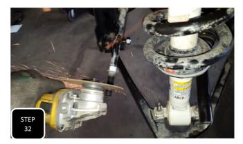
**Step 32** Mark a line 9/16" in from the threaded end of the inner tie rod and cut this section off. **NOTE: MAKE SURE TO CLEAN UP THE END SO THAT THE OUTER TIE ROD CAN THREAD BACK ON PROPERLY.**
