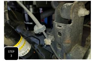
**Step 3** Unclip the ABS line guide clips from the back side of the upper control arm mounts on both sides.
