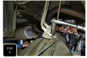
**Step 6** Unbolt the brakeline bracket from on top of the diff to allow for more slack when installing the coil spacers.
