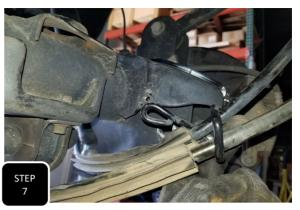
**Step 7** Locate the E-brake cable guide brackets on the frame in the passenger side wheel well and at the driver's side lower control arm mount on the axle. Unbolt both and completely remove the pass side bracket from E-brake cable.
