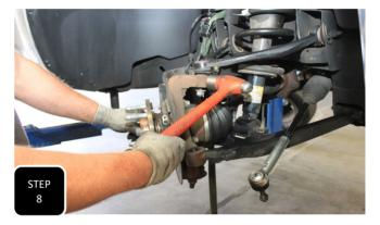
**Step 8** Loosen the upper ball joint nut, but do not remove. Hit the side of the spindle, right at the ball joint, with a hammer to break the ball joint loose. The nut will catch the spindle.
