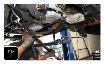
**Step 14** Unbolt the 4 bolts attaching the sway bar to the frame and remove the sway bar. **NOTE: TAKE NOTE THAT THE ENDS OF THE SWAY BAR SWOOP UPWARD. YOU WILL FLIP THIS OVER SO THEY SWOOP DOWNWARD WHEN THE SWAY BAR IS RE-INSTALLED.**
