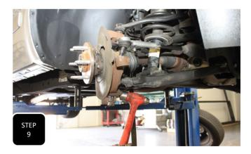
**Step 9** Loosen the lower ball joint nut, but do not remove. Next, hit the side of the spindle, right at the nut, with a hammer to break the ball joint loose. The nut will catch the spindle.
