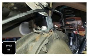
**Step 21** Remove the "O" ring that is on the factory mounting bolt for the brake line bracket at the top of the diff. Next, attach the provided brake line bracket to the top of the diff using this bolt and tighten.
