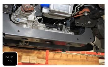
**Step 16** Loosely install the rear subframe using the factory hardware. The notch in the vertical rise of the subframe goes on the driver's side, facing forward to allow for clearance with the diff.
