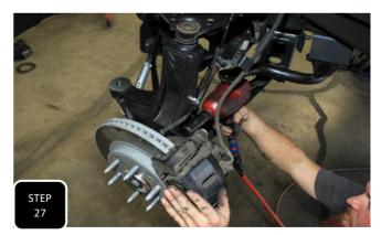
**Step 27** Unbolt the factory bracket that attaches the brakeline to the frame to gain extra slack in the line. Next, attach the brake caliper to the steering knuckle using the factory bolts and tighten.
