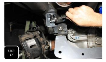
**Step 17** Install the sway bar drop down brackets using the supplied M10 bolts and washers. The open end of the bracket will face the inside of the truck and the bracket needs to swoop towards the rear of the truck.
