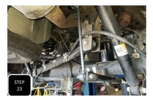
**Step 23** Install the new, longer sway bar end links using the factory bolt at the frame and the provided 12mm bolt at the sway bar, then tighten.
