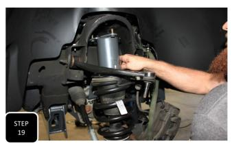
**Step 19** Locate the two struts and attach the strut spacer to the top using the factory nuts. Next, loosely install both sides using the provided nuts. **NOTE: THE SPACERS WILL ONLY FIT ONE WAY AND DO NOT FULLY TIGHTEN THE NUTS AT THE FRAME AT THIS TIME.**
