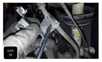
**Step 29** There is a mounting bracket on the middle of the soft brake line that needs to be removed. Very carefully, cut a groove in the bracket where it wraps around the line. This will create a weak spot so you can use a flat head screw driver to pry the bracket open and remove it. **NOTE: BE VERY CAREFUL NOT TO CUT ALL THE WAY THROUGH THE BRACKET OR CUT THE LINE ITSELF.**
