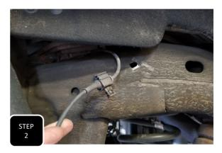
Step 2 Separate the ABS guide clip, on each side, from the frame to allow for more slack during the install.
