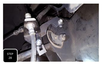
**Step 28** Locate the new brakeline mounting bracket and attach it to the side of the coil bucket using the factory brakeline bracket mounting bolt. Next, attach the factory brakeline bracket to the new brakeline bracket using the provided 8mm bolt, nut, and washers.
