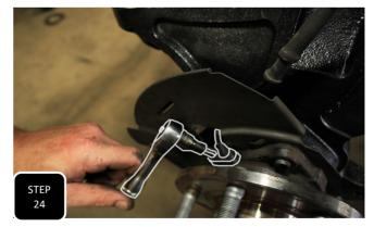
**Step 24** Unclip the ABS line from the frame, right next to where the brake line goes from soft to hard line. Next, use the extra slack gained to guide the ABS sensor down the steering knuckle and attach it to the wheel bearing using the factory bolt.
