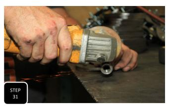
**Step 31** Remove the outer tie rod from the inner tie rod and mark a line 1/2" from the end of the threaded hole and cut this 1/2" section off. **NOTE: MAKE SURE YOUR CUT IS STRAIGHT SO THAT THE JAM NUT TIGHTENS UP PROPERLY.**
