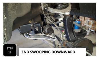
**Step 18** The ends of the sway bar originally swooped upward. The sway bar will now get re-installed with the ends swooping downward, the opposite of how they were. Use the factory bolts along with the provided nuts and washers to attach the sway bar to the drop down brackets and tighten.
