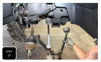
**Step 13** Unbolt both lower control arm mounting bolts and remove the lower control arm. Repeat steps 1-15 on the other side.
