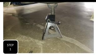
**Step 1** Jack up the rear of the truck and support under the frame rails with jack stands. Keep an adjustable jack under the diff for height adjustment.
