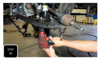
**Step 20** Loosely attach both lower control arms using the provided 5/8" hardware and then swing the arms up and loosely attach them to the bottom of the strut using the factory hardware. **NOTE: DO NOT FULLY TIGHTEN THE LOWER CONTROL ARM BUSHINGS UNTIL THE TRUCK IS BACK ON THE GROUND AT RIDE HEIGHT.**
