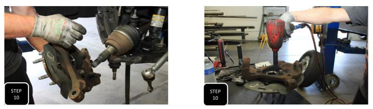
**Step 10** Remove the spindle and set it face down on the wheel studs. Next, remove all 3 bolts attaching the wheel bearing to the spindle and separate the two.
