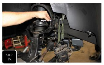
**Step 25** Using the provided loom clamps and factory 6 mm bolts, guide and attach the ABS line up the back side of the neck of the steering knuckle and to the upper control arm.
