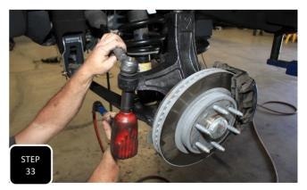
**Step 33** Once both ends are trimmed down, thread them back together and attach the tie rod to the steering knuckle using the factory nut.
