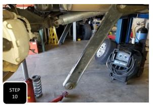
**Step 10** Make sure the adjustable jack under the diff has a provision to keep the diff from rotating, then unbolt both lower link arms from the axle, loosen the bolts at the frame, and allow them to both drop down, away from the axle. **NOTE: IF THE PINION IS NOT SUPPORTED, THE DIFF WILL WANT TO ROTATE DOWN.**
