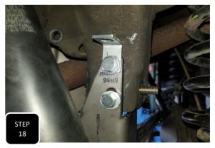
**Step 18** Re-install the bracket using the provided zinc plated crush tube and 14mm hardware. Next, install the provided 7/16" bolts, nuts, and washers through the two side holes. You will also be attaching the provided pass side ABS line bracket to the upper bolt with the "D" shaped hole facing upward, then tighten all 3 bolts.
