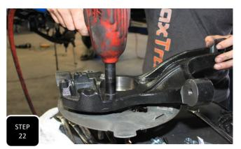
**Step 22** Place the factory hub assembly along with the factory dust shield onto the new steering knuckle and then flip the assembly over and attach the two together using the factory bolts and tighten.
