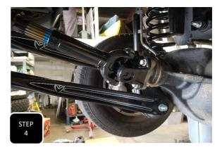
**Step 4** Using retainer clip pliars, spread open the retainer clip in the new drive flange and slide the drive shaft onto the transfer case output shaft and make sure the clip engauges in the groove. Next, attach the other end of the drive shaft to the front differential using the factory bolts and torque to 60 ft/lbs
