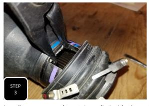
**Step 3** Slide the boot out of the way and using a set of retainer ring pliers, open up the retainer clip inside the notch of the drive shaft and remove the drive shaft.
