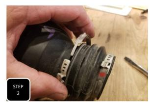
**Step 2** Using a flat head screw driver, open up and separate the CV style clamps attaching the dust boot over the coupler joint attaching the driveshaft to the transfer case.
