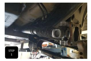
**Step 1** Unbolt and remove the 4 bolts that attach the front driveshaft to the front differential and separate.
