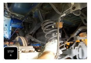
**Step 4** Lower the axle and remove both rear coils. NOTE: BE CAUTIOUS NOT TO STRETCH OR DAMAGE ANY BRAKE LINES OR ABS LINES.
