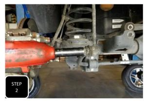
**Step 2** Unbolt both sway bar endlinks at the sway bar and separate.
