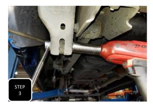
**Step 3** Apply a little bit of pressure to the differential with the jack and then unbolt both shocks at the axle and separate.
