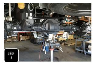
**Step 1** Jack up the rear of the vehicle and support under the frame rails with jack stands. Keep an adjustable jack under the differential for height adjustment.
