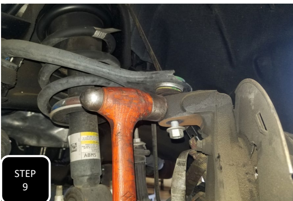
Step 9 Brake each ball joint loose by hitting the side of the spindle with a hammer, right at the ball joint. The nut will catch the spindle, then remove the spindle.
