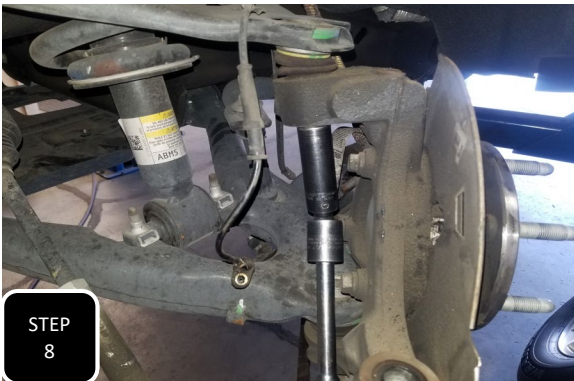
Step 8 Loosen both the upper and lower ball joint nuts, but do not remove.
