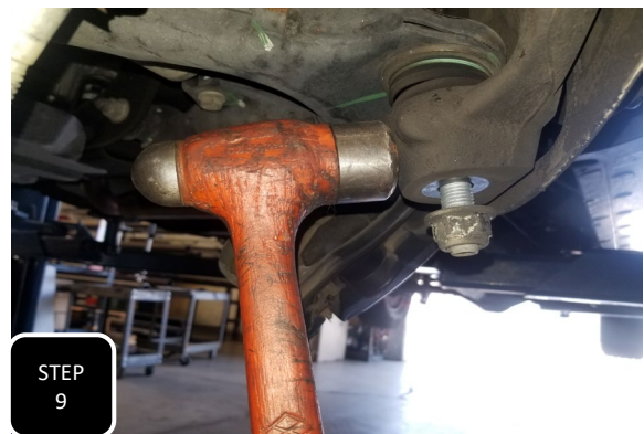
Step 9 Brake each ball joint loose by hitting the side of the spindle with a hammer, right at the ball joint. The nut will catch the spindle, then remove the spindle.
