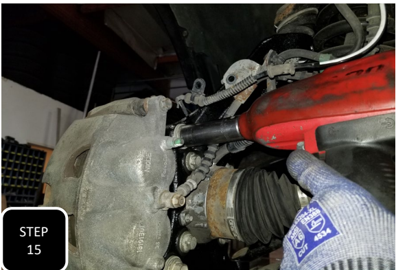
Step 15 Re-install the brake caliper using the factory bolts and tighten.
