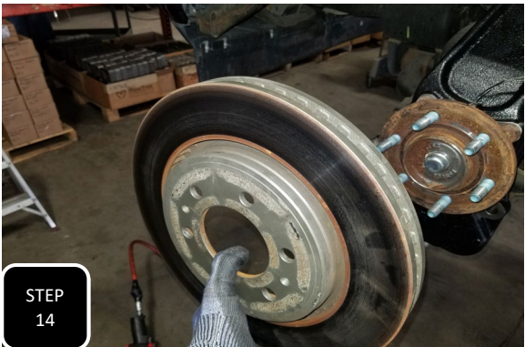
Step 14 Loosely install the brake rotor by sliding it onto the wheel studs.
