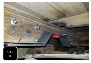
**Step 8** First, install supplied bump stop onto the hole at the center of the C-notch. Next, using the supplied 1/2" hardware, attach the frame support to the frame and torque the bolts to 65 ft/lbs.
