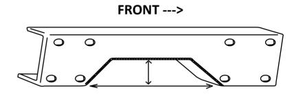
**Step 6** Check for proper fitment and clearance as needed until the frame support fits flush to the frame. The longer, rectangular 4 bolt pattern goes towards the front of the truck and the square, 4 bolt pattern towards the rear.
