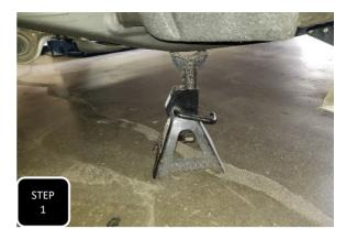
**Step 1** Jack up the rear of your vehicle and support under the frame with jack stands. Allow the suspension to extend to full droop and remove the wheels. **NOTE: IT IS RECOMMENDED TO INSTALL THE FLIP KIT FIRST SO THAT YOU CAN MARK WHERE THE CENTER OF THE AXLE WILL CONTACT THE FRAME.**
