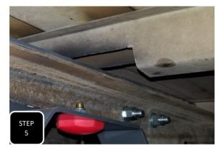
**Step 5** Before being able to test fit the frame support, you will need to trim the bed rib, directly above, in order for the frame support to be able to slide over the top of the frame. Using a suitable cutting device, trim the bed rib about 1/2" up from the bottom. Trim from the end of the rib to at least the inside edge of the frame to ensure an easy install of the frame support and no contact of the two.
