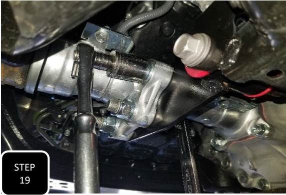
Step 19 Torque all 7 diff mounting bolts to 80 ft/lbs.
