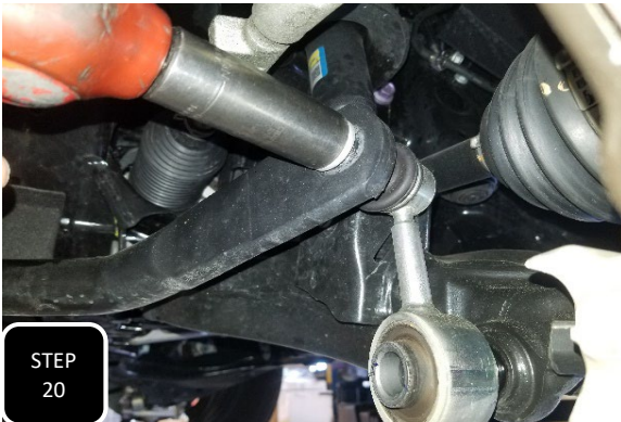
Step 20 Lower the truck down to the ground and re-install the sway bar end links using the factory hardware. NOTE: HAVING THE TRUCK ON THE GROUND AT RIDE HEIGHT MAKES INSTALLING THE SWAY BAR ENDS LINKS MUCH EASIER.
