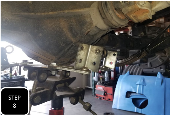
Step 8 Make sure the adjustable jack under the diff has a provision to keep the diff from rotating, then unbolt both lower link arms from the axle, loosen the bolts at the frame, and allow them to both drop down, away from the axle. NOTE: IF THE PINION IS NOT SUPPORTED, THE DIFF WILL WANT TO ROTATE DOWN.
