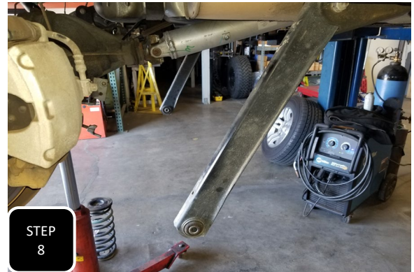
Step 8 Make sure the adjustable jack under the diff has a provision to keep the diff from rotating, then unbolt both lower link arms from the axle, loosen the bolts at the frame, and allow them to both drop down, away from the axle. NOTE: IF THE PINION IS NOT SUPPORTED, THE DIFF WILL WANT TO ROTATE DOWN.
