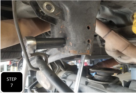
Step 7 Unbolt the trac bar from the mount on the frame and separate.
