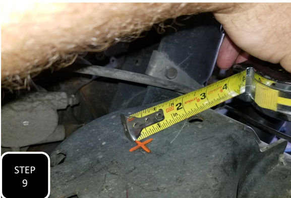
Step 9 Locate the bump stop striker pads on the axle, then measure and mark an "X" 2 1/8" straight forward from the existing hole in the plate. Next, drill a 1/2" hole through your mark. NOTE: CHECK THE FACTORY HOLE FOR WELD SLAG. IT MAY NEED TO BE CLEANED OUT TO ACCEPT A BOLT.
