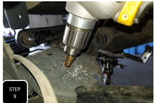
Step 9 Locate the bump stop striker pads on the axle, then measure and mark an "X" 2 1/8" straight forward from the existing hole in the plate. Next, drill a 1/2" hole through your mark. NOTE: CHECK THE FACTORY HOLE FOR WELD SLAG. IT MAY NEED TO BE CLEANED OUT TO ACCEPT A BOLT.
