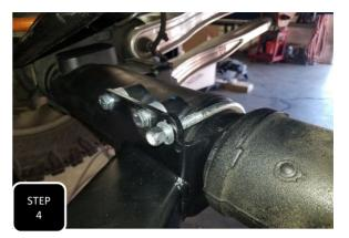
**Step 4** Slide the supplied 4.250" U-bolt around the axle housing and through the slotted holes in the center mounting bracket, then start the nuts/washers.
