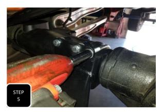
**Step 5** Now that all of the mounting hardware is started, tighten down the four M10 bolts to 30 ft/lbs and then the U-bolt to 80 ft/lbs.
