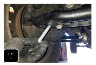
**Step 1** Unbolt and remove the two bolts attaching the factory steering stabilizer to the tie rod. **NOTE: SAVE THESE BOLTS FOR RE-INSTALLATION.**
