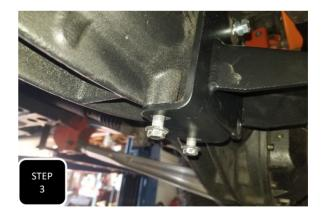
**Step 3** Loosely attach the new, center mounting bracket to the middle of the axle using the provided M10 bolts, washers, and aluminum spacers at the upper factory holes. Next, loosely install two of the factory bolts into the the lower mounting holes. **NOTE: THE SPACERS GO BETWEEN THE AXLE AND BRACKET.**
