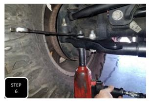
**Step 6** Attach the passenger side mounting plate to the tie rod using the factory bolts. Make sure the stabilizer mounting tab swoops downward and torque the bolts to 65 ft/lbs.
