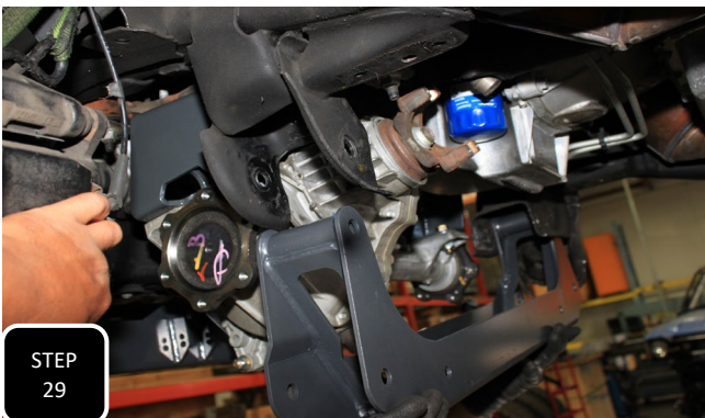
Step 29 Loosely install the rear subframe using the factory hardware. The notch in the vertical rise of the subframe goes on the driver's side, facing forward to allow for clearance with the diff.
