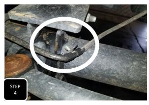
**Step 4** Unclip the hub vacuum line from the top of the driver's side radius arm. Next, Unclip the hub vacuum line from the side of the bump stop striker plate on the passenger side of the axle.
