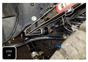
**Step 34** Torque the trac bar bolt at the frame to 406 ft/lbs.
