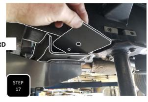
**Step 17** Locate the flat plate labeled DS and slide it into the cross member above the back of the 4 link bracket. Line up the holes and loosely attach the plate and bracket together using the provided M12" and 5/16" socket head allen bolts. Once all of the bolts have been installed, torque the large, M18 bolt to 200 ft/lbs and the M12 socket head allen bolt to 55 ft/lbs. **NOTE: THE DRIVER'S SIDE IS THE LONGER PLATE**
