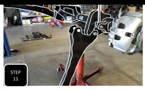
**Step 11** Loosen all 3 radius arm bolts, one side at a time. Then remove the upper bolt at the axle and the bolt at the frame and pivot the radius arm down out of the way. **NOTE: WORK ON ONE SIDE AT A TIME SO THAT THE AXLE IS SAFELY SUPPORTED AT ALL TIMES.**
