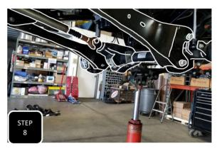
**Step 8** Once both sides have the coils removed and are supported by the new shocks, move the adjustable jack to the middle of the axle and apply pressure.
