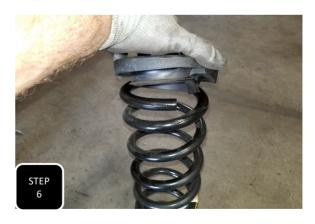
**Step 6** Lower down the axle and remove the coil. Separate the rubber isolator and save for use on the new coils. **NOTE: TAKE CARE NOT TO DAMAGE THE BRAKE LINE OR ABS LINE.**
