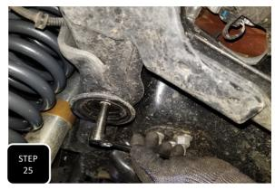
**Step 25** Pry the factory bump stop out of its mounting cup on the frame and then remove the single mounting bolt and mounting cup.
