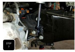
**Step 7** Loosely attach the new shock to hold the axle, then move the jack to the passenger side and repeat steps 5-7. **NOTE: THE SHOCKS WILL HOLD THE AXLE AS YOU MOVE THE JACK AND CONTINUE THROUGH THE INSTALL.**
