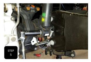
**Step 5** Move the adjustable jack to the driver's side and apply pressure to the axle. Next, unbolt the driver's side shock at both ends and remove.
