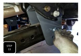
Step 13 Swing the radius arm up and attach it to the new bracket using the provided M18 bolt.
