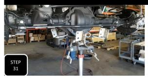
**Step 31** Jack up the rear of the truck and support under the frame rails with jack stands. **NOTE: KEEP AN ADJUSTABLE JACK UNDER THE AXLE FOR HEIGHT ADJUSTMENT.**
