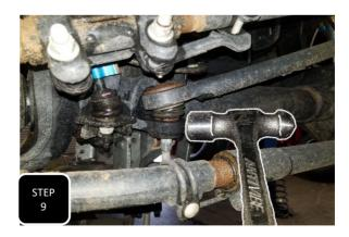
**Step 9** Unbolt the nut attaching the trac bar to the axle and break the joint loose by hitting the side of the axle hole with a hammer. **NOTE: NEVER HIT A ROD END ON THE THREADS.**
