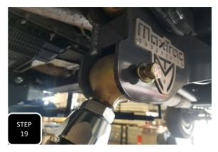
**Step 19** Locate the other arm that matches the one you just installed, adjust it to an eye-eye length of 32 1/2" and grease the rod end. Next, loosely install it into the bottom hole of the 4 link frame bracket using the provided 9/16" bolt, washers, and nut. **NOTE: THE ROD ENDS ARE NOT PRE-GREASED AND REQUIRE GREASE FOR PROPER FUNCTION.**
