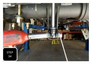
Step 34 Install your new longer shocks using the factory hardware and tighten. NOTE: MAX TRAC SHOCKS HAVE TO BE MOUNTED WITH THE BODY OF THE SHOCK AT THE AXLE AND THE SHAFT OF THE SHOCK AT THE FRAME. FOX SHOCKS WILL BE MOUNTED THE OPPOSITE OF THIS.
