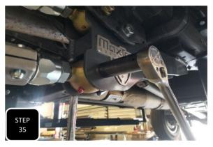
**Step 35** If you installed the MaxTrac 4 links, torque the axle side bolts to 200 ft/lbs and the frame side bolts to 100 ft/lbs. If you purchased the radius arm bracket kit then torque all 6 radius arm bolts to 200 ft/lbs.
