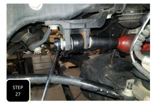
**Step 27** Loosely attach the new, adjustable trac bar to the frame using the factory bolt and only snug up the bolt. **NOTE: THIS BOLT WILL NOT GET FULLY TIGHTENED UNTIL THE TRUCK IS BACK ON THE GROUND AT RIDE HEIGHT.**
