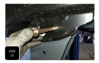
**Step 12** Install the radius arm drop down bracket into the factory radius arm bracket on the frame and loosely attach it using the factory bolt at the big hole and the provided small machined washers along with the provided 9/16" bolt at the small hole. **NOTE: THE SMALL MACHINED WASHERS GET INSTALLED FROM THE OUTSIDE OF THE BRACKET FACING INWARD.**
