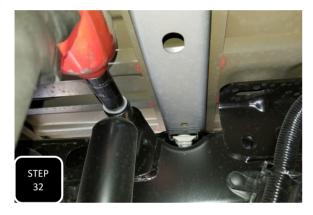
**Step 32** Unbolt both rear shocks at both ends and remove.
