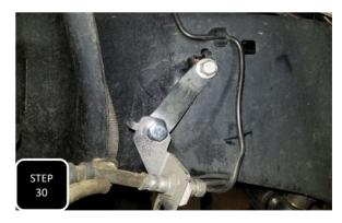
**Step 30** Attach the passenger side, shorter bracket to the passenger side frame hole using the factory bolt. Next, gently unravel the factory hardline until the factory bracket reaches the new mounting hole on the provided bracket and attach the two using the provided M8-1.25 x 20mm bolt, nut, and washers.
