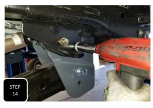
**Step 14** Repeat steps 11-13 on the driver's side and then tighten the bolts attaching the bracket to the frame, the big bolt gets torqued to 200 ft/lbs and the smaller one to 130 ft/lbs. The radius arm bolts will not get tightened until the truck is on the ground at ride height.
