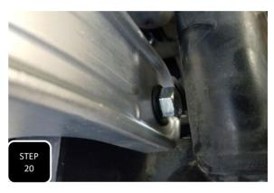
**Step 20** Insert the larger machined sleeves into the "upper" link arm hole at the axle side of the link. Both sleeves get installed from the outside facing inward then attach the link to the axle using the provided M18 bolt, nut and washers.
