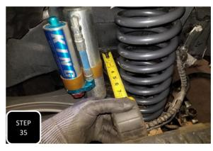
**Step 35** Install the wheels and tires then lower the truck back down to ride height. Drive the truck backwards about 10 feet and then forward about 10 feet to settle the suspension. Next, take a measurement from the inside of the front tire to the frame on both sides (in a consistant spot) and then compare your measurements.
