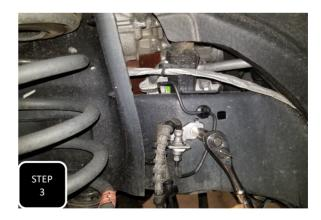
**Step 3** Unbolt the brake lines from the frame at both sides and un-ravel the hard brake line a little bit. **NOTE: THIS WILL ALLOW FOR SLACK IN THE LINE WHEN THE COILS ARE REMOVED.**
