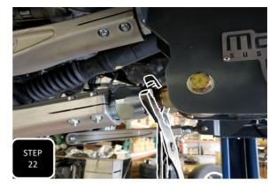
**Step 22** Tighten down all 4 of the M8 pinch bolts and then cinch down the two jam nuts on the rod ends.
