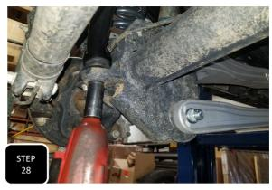
**Step 28** Loosen the adjustment collar of the trac bar and adjust the length until the rod end drops into the mounting hole on the axle. Next, torque the nut to 200 ft/lbs. **NOTE: FINAL ADJUSTMENTS WILL BE MADE WHEN THE TRUCK IS BACK ON THE GROUND AT RIDE HEIGHT.**
