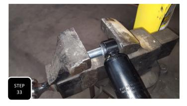
**Step 33** If installing Max Trac or Vulcan series shocks, you will need to grease the bushings and use a bench vise to press in the shock sleeves.
