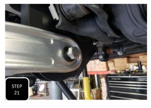
**Step 21** Remove the upper bolt attaching the radius arm on the other side so that the axle can be rotated. Next, insert two of the larger sleeves into the hole in the "lower" link and attach the lower link to the axle using the provided M18 bolt, nut, and washers. **NOTE: DO NOT FULLY TIGHTEN THESE BOLTS UNTIL THE TRUCK IS BACK ON THE GROUND AT RIDE HEIGHT.**
