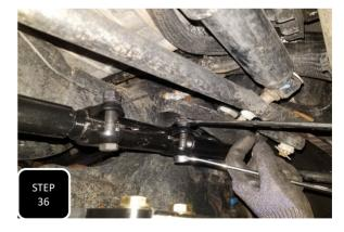
**Step 36** Loosen up the adjustment clamps on the trac bar and adjust the trac bar accordingly until your measurements match each other. Next, tighten down both clamps on the collar.
