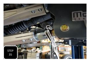
Step 35 Tighten down all 4 of the M8 pinch bolts and then cinch down the two jam nuts on the rod ends. REPEAT STEPS 21-32 ON THE OTHER SIDE.
