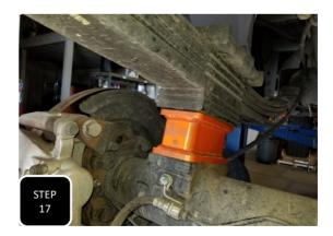
**Step 17** Install the new lift block. The block is flat so it can be installed either way. Align the center pins and jack up the axle to seat the block.
