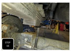
**Step 16** One side at a time, loosen both U-bolts, remove the U-bolts, and lower the axle to make room for the lift block. **NOTE: IT WILL HELP THE ALIGNMENT OF THE LIFT BLOCK TO SLIGHLY LOOSEN THE U-BOLTS ON THE OTHER SIDE.**
