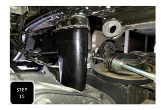
**Step 15** Locate the new, longer bump stops and spray the top of them with grease to make them easier to install. Next, line them up, one at a time, and using the jack under the axle as a press, jack the axle up until the bump stop presses into the cup all of the way.
