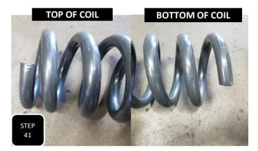
**Step 41** Place the rubber isolator on top of the new coil and install the coil. Make sure the nipple on the isolator aligns with the hole in the coil bucket then jack up the axle so that pressure is applied and re-attach the shock. **NOTE: THE COIL NEEDS TO BE INSTALLED WITH THE FLATTER SIDE FACING UPWARD AND THE PART # RIGHT SIDE UP.**
