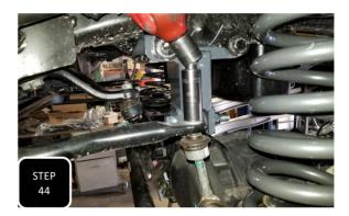
**Step 44** Attach the sway bar to the drop down brackets and to the axle using the provided hardware at the brackets and the factory nuts at the axle then tighten them all down. **NOTE: IT WILL EASE THE INSTALL TO FIRST LOOSELY ATTACH THE SWAY BAR TO THE END LINKS AND THEN TO THE BRACKETS ON THE FRAME.**
