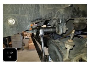
**Step 11** Remove the bolt attaching the trac bar to the bracket on the frame and separate. Allow the trac bar to rest on the axle.
