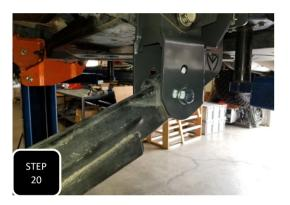
Install the radius arm into the: Upper hole for the 4" lift Lower hole for the 6" lift.
