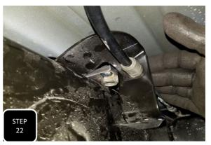
**Step 22** Insert the provided 9428RAB-2 nut plate on top of the frame, behind the E-brake bracket with the notched edge facing the front of the truck and the nut towards the outside of the frame facing downward. **NOTE: THIS E-BRAKE BRACKET IS ONLY ON 2021 AND NEWER TRUCKS.**
