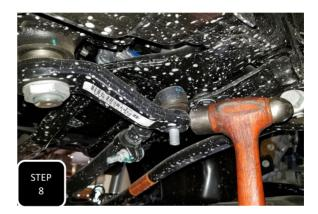
**Step 8** Remove the nut attaching the drag link to the pitman arm then brake the drag link loose by hitting the side of the pitman arm with a hammer, right at the joint, then separate. **NOTE: NEVER HIT THE THREADS OF THE ROD END.**
