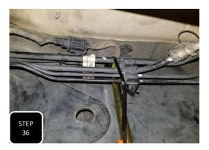
**Step 36** Use the supplied zip tie to attach the fuel line assembly to the U-bolt.
