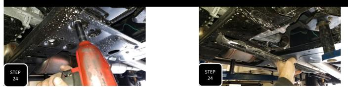
**Step 24** Unbolt and remove the skid plate under the transfer case and set aside to be re-installed later.
