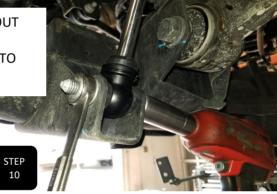
**Step 10** Install the new shocks and tighten down both ends. **NOTE: DO NOT OVER TIGHTEN THE TOP BUSHING OF THE SHOCK OR THE BUSHING WILL NOT BE ABLE TO FLEX AND COULD DAMAGE TO THE SHOCK.**
