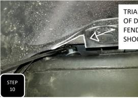
TRIANGULAR NOTCH CUT OUT OF DRIVER'S SIDE PLASTIC FENDER WELL FOR ACCESS TO SHOCK MOUNT.
