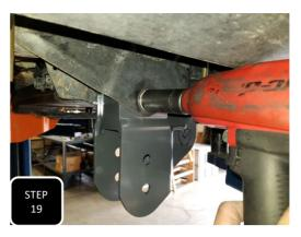
**Step 19** Loosely install the new radius arm bracket into the factory mount using the factory radius arm bolt in the main hole and the supplied hardware for the U-bolt. Push the bracket up tight against the frame and tighten the U-bolt first, then tighten the stock mounting bolt. Once tight, torque the factory bolt to factory specs and the U-bolt to 100 ft/lbs.
