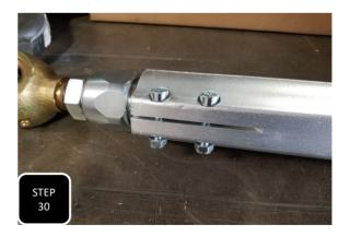
**Step 30** Get all 4 link arms in front of you with all of the Max Trac logos facing in the same direction and the two holed pinch seem facing up. Loosely install the provided M8 socket head bolts with the head of the bolt on the same side as the top of the Max Trac logo.
