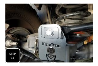
**Step 11** Use a rachet strap to pull the axle over and align the trac bar with the hole in the new bracket then loosely attach with the provided square plates and M14 bolt. The off-center hole will get installed with the bolt towards the driver's side for the 4" and 6" lift. Its only off-set to the pass side for the 8" lift. **NOTE: DO NOT TIGHTEN UNTIL THE TRUCK IS ON THE GROUND AT RIDE HEIGHT.**
