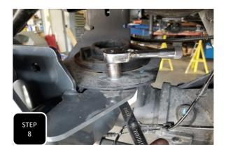
**Step 8** Tighten up the two 3/8" bolts. **NOTE: THE EASIEST WAY TO TIGHTEN DOWN THE BOTTOM 3/8**" **BOLT IS TO STICK A FLAT HEAD SCREW DRIVER DOWN INSIDE THE BRACKET AND WEDGE IT AGAINST THE HEAD OF THE BOLT WHILE TIGHTENING THE NUT WITH A RATCHET.**
