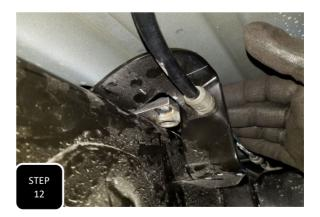
**Step 12** Insert the provided 9428RAB-2 nut plate on top of the frame, behind the E-brake bracket with the notched edge facing the front of the truck and the nut towards the outside of the frame facing downward. **NOTE: THIS E-BRAKE BRACKET IS ONLY ON 2021 AND NEWER TRUCKS.**
