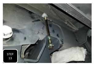
**Step 13** Models without the welded on brake line will look like this to where the nut plate will openly sit on top of the frame.
