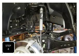
**Step 4** Completely remove the driver's side shock and loosely install the new shock as support for the axle while you are installing the lift. Next, repeat steps 3-4 on the passenger side and then move the jack back to the driver's side.
