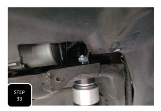
**Step 33** Move the jack to the driver's side of the axle and apply pressure. Remove the nut at the top of the shock and lower the axle to make room for the new coil.
