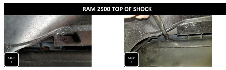
**Step 3** The top of the shock on Ram 2500's is a standard stem that is hidden behind the plastic wheel well liner. Using a knife, cut a clean opening for access to the stem nut and remove the shock.
