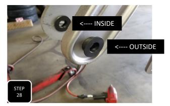
**Step 28** Loosely attach both links to the 4link bracket first using the provided 9/16" bolts and then install the provided machined, hat looking, sleeves on the other end of the link with 1 hat inside the clevis and 1 hat on the outside.
