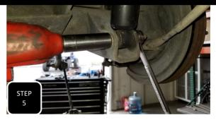
**Step 5** Install the new shocks and tighten using factory hardware at the bottom. **NOTE: MAXTRAC SHOCKS ARE A TWIN TUBE SHOCK THAT NEEDS TO BE FULLY CYCLED BEFORE INSTALL SO FULLY COMPRESS THEM & LET THEM REBOUND ABOUT 2-3 TIMES.**
