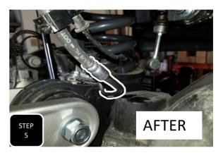
**Step 5** Locate where the brake line goes from soft line to hard line on the axle and gently bend the hardline upward so that it is at about a 45 degree angle to allow for more slack in the line.
