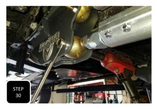
**Step 30** Tighten down the frame side bolts of the links completely and the axle side only hand tight. The axle side will get fully tightened when the truck is back on the ground at ride height. Torque the rod end bolts to 100 ft/lbs.
