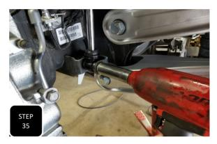
**Step 41** Repeat steps 33-34 on the other side and then tighten the top and bottom of both shocks.
