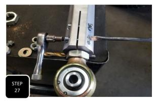
**Step 27** The upper links will not require any further adjustment so tighten down the pinch bolts now. Use a flat head screw driver, wedged between the nut and wall of the hole, to hold the nut from spinning. **NOTE: THE GAP BETWEEN THE UPPER ARM AND FRAME WILL BE VERY TIGHT AND MAKE IT VERY DIFFICULT TO TIGHTEN THESE PINCH BOLTS AFTER THE ARM IS INSTALLED.**
