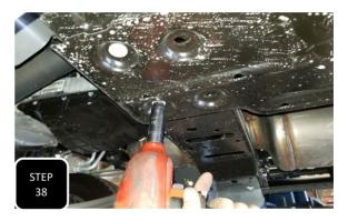
**Step 38** Re-attach the brake line brackets to the top of the axle and ensure that the brake lines are not tight when the suspension is at full droop. Next, re-install the skid plate under the transfer case and tighten.
