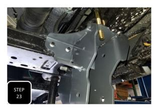
**Step 23** Locate the appropriate side 4link bracket so that when installed the Max Trac logo faces outward and the 2 holed side bracket faces inward. Loosely install the bracket using the factory radius arm bolt at the main hole, slide the two cross member bolts forward, and align the U-bolt with the top holes.
