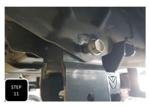
Step 11 Loosely install the radius arm drop down bracket using the factory bolt.
