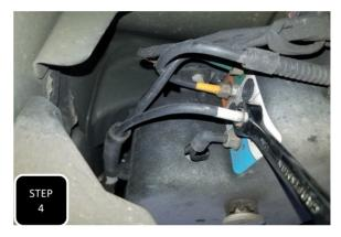
**Step 4** Locate the air ride valve block on the outside of the passenger side frame rail and crack open the two lines leading to the rear air bags to bleed the air out of them. Once the bags have been deflated, tighten up both fittings.
