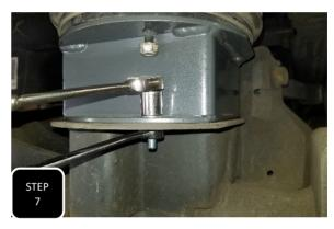
**Step 7** Tighten down the studs at the air bags using the factory nuts. Next, attach the spacers to the axle using the provided M8 bolts, nuts and washers then tighten.
