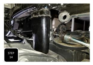
**Step 14** Locate the new, longer bump stops and spray the top of them with grease to make them easier to install. Next, line them up, one at a time, and using the jack under the axle as a press, jack the axle up until the bump stop presses into the cup all of the way.
