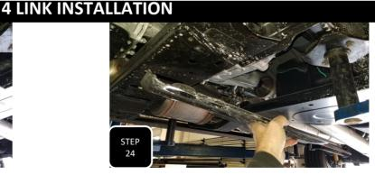
**Step 24** Unbolt and remove the skid plate under the transfer case and set aside to be re-installed later.
