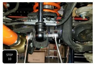
**Step 10** Once the mounting hardware has been installed, install the shocks on the truck using the factory bolts top and bottom. Torque bolts to 55 ft/lbs.
