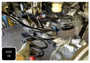
**Step 19** Lower down the axle and remove both coil springs.
