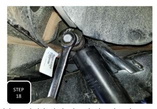
**Step 18** Apply some pressure to the rear axle with the jack and then unbolt both shocks at both ends and remove.
