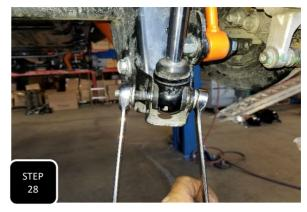
**Step 28** Once the mounting hardware has been installed, install the shocks on the truck using the factory bolts top and bottom. Torque bolts to 55 ft/lbs.
