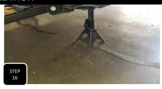
**Step 16** Jack up the rear of the truck and support under the frame with jack stands. Keep an adjustable jack under the differential for height adjustment.
