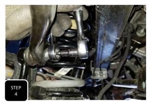
**Step 4** Unbolt both front sway bar end links at both ends and remove.
