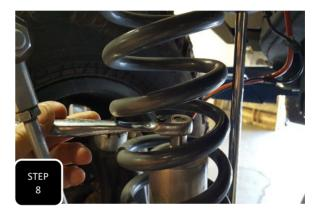
**Step 8** Drop the supplied 7/16" bolt and washer into the bumpstop and tighten down to 45 ft/lbs.
