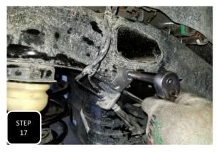
**Step 17** Working on both sides at the same time, unbolt the brake line guide bracket from the frame and pull down the hard line a little bit to gain slack in the line.
