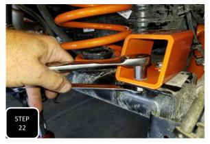
**Step 22** Attach the new bump stop extensions to the axle using the provided 3/8" hardware. The extensions will need to off-set towards the front of the truck.
