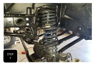
**Step 7** Locate the new front coil springs and aluminum bump stop extensions. Hold the bump stop extensions inside the coils and install the springs onto the truck.
