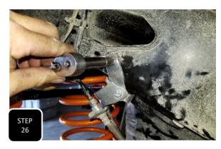
**Step 26** Locate the brake line extension brackets and attach them with the bent tab facing down, inward, and towards the front of the truck. Loosely install them using the factory mounting bolt. Next, attach the factory bracket to this bracket using the provided 1/4" hardware. Rock both brackets forward so the tab on the new bracket hits the frame and the tab on the factory bracket hits the new bracket and tighten both bolts.
