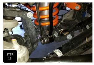
**Step 13** Install the factory rear sway bar end links on the front using the factory hardware.
