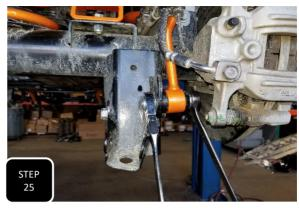
Step 25 Attach the new sway bar end links to the sway bar using the supplied M12 hardware and to the axle using the factory M12 hardware. The links will need to go wider at the sway bar. Next, torque the bolts to 50 ft/lbs. NOTE: THE DRIVER'S SIDE END LINK WILL CONTACT THE WHEEL, IF STOCK WHEELS ARE INSTALLED, ONLY AT FULL SUSPENSION DROOP, BUT NOT DURING NORMAL DRIVING.
