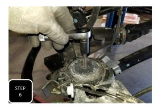
Step 6 Lower the axle and remove both front coil springs. Next, using a 7/16-14 tap, thread the center hole in the coil guide on the axle.
