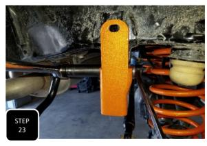
**Step 23** Unbolt the trac bar from the mount at the frame and separate. Loosely attach the new trac bar bracket using the supplied M14 hardware and zinc plated crush tube. The new bracket will fit around the factory bracket.
