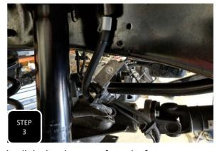
**Step 3** Unbolt both front brake line brackets from the frame and pull the bracket away from the frame.
