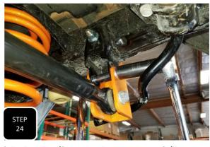
**Step 24** Install the supplied  $1/2 \times 5 \cdot 1/2$ " bolt through the side of the bracket/frame and torque to 85 ft/lbs. Next, loosely attach the trac bar to the new bracket using the factory hardware, but do not tighten at this time. Tighten the bolt through the original trac bar hole and torque to 100 ft/lbs.
