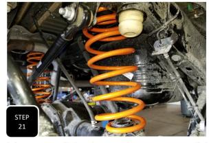
**Step 21** Install the new coil spacers on the lower coil mount and then re-install the plastic isolator. Next, install the new springs and jack up the axle until both springs are properly seated.
