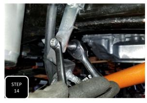
**Step 14** Locate the brake line extension brackets and loosely attach them to the frame using the factory bolts. The bent tab will face out, away from the frame. Next, attach the two brackets together using the provided 1/4' hardware and rotate the brackets until the bent tab on the factory bracket touches the new bracket, and tighen. Lastly, tighten the bolt at the frame.
