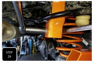
**Step 29** Install the wheels and tires then lower the truck down to ride height. Jump on the rear bumper a few times to settle the rear suspension then torque the trac bar bolt to 100 ft/lbs.
