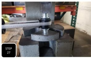
**Step 27** Locate the new rear shocks and press in the provided hardware. The top hardware consists of two sleeves with a rib in the middle and the bottom sleeve is just a straight sleeve. First grease the bushings and then press in the sleeves using a bench vise or arbor press.
