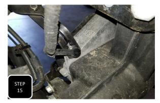
**Step 15** Re-attach both wire clips for the front differential wiring and then move to the rear of the vehicle.
