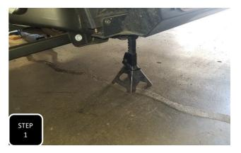
**Step 1** Jack up the front of the vehicle and support under the frame with jack stands. Keep an adjustable jack under the axle for height adjustment.
