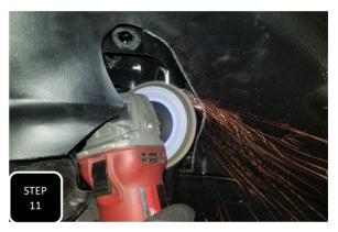
**Step 11** If installing Vulcan Series reservoir shocks, some vehicles may run into a contact issue between the 90 degree reservoir fitting and the factory shock tower. Mark the contact area and then clearance, as needed, using a suitable grinder. Last, seal up the ground area with some black spray paint to avoid rust.
