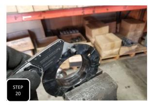
**Step 20** Remove the plastic lower coil isolator and cut off the guide nipple using a suitable cutting device.
