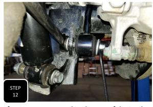
**Step 12** Your factory rear sway bar end links will get used in the front so now proceed to the rear of the truck and remove both factory sway bar end links.
