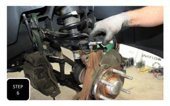
**Step 6** Unbolt the ABS sensor from the hub assembly and then the guide bracket from the top of the spindle. Support the ABS sensor out of the way so that it does not get damaged during the install.
