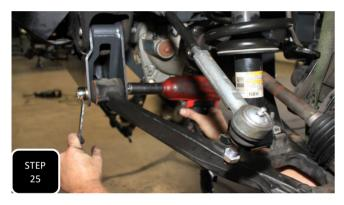
**Step 25** Now that the suspension is settled and the vehicle is sitting at ride height, go back and tighten all of the bolts that were left loose. **NOTE: TIGHTENING THE CONTROL ARM BUSHINGS AND DIFFERENTIAL WHILE THE TRUCK IS AT RIDE HEIGHT WILL ENSURE THE DIFF IS CENTERED AND PROLONG THE LIFE OF THE BUSHINGS.**
