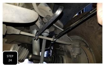
**Step 24** Install the new wheels and tires, then move the truck forward and back about 10 feet while moving the steering back and forth to settle the suspension. Next, adjust the vehicles toe alignment close to straight so that the vehicle is safe to drive to the alignment shop.
