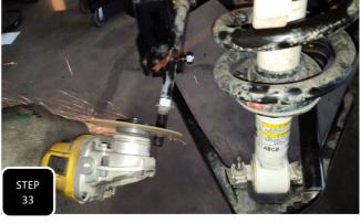
Step 33 Mark a line 9/16" in from the threaded end of the inner tie rod and cut this section off. NOTE: MAKE SURE TO CLEAN UP THE END SO THAT THE OUTER TIE ROD CAN THREAD BACK ON PROPERLY.
