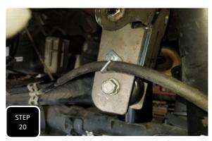
**Step 20** Slide the E-brake guide bracket onto the E-brake cable near the trac bar bracket on the passenger side and then attach this bracket to the small hole on the back of the trac bar bracket using the provided 8mm bolt nut and washers. **NOTE: DO NOT FULLY TIGHTEN THIS BRACKET. ONLY SNUG IT UP AS IT WILL NEED TO PIVOT AS THE SUSPENSION CYCLES.**
