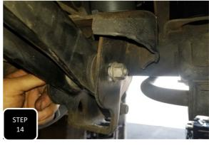
**Step 14** Loosely re-attach the lower control arm to the axle and only snug up the nuts. **NOTE: THESE BOLTS WILL GET FULLY TIGHTENED WHEN THE TRUCK IS BACK ON THE GROUND AT RIDE HEIGHT.**
