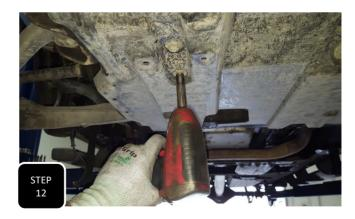
**Step 12** Unbolt and discard the plastic skid plate that covers from the bumper to the rear cross member of the lower control arms.
