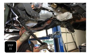
Step 15 Unbolt the 4 bolts attaching the sway bar to the frame and remove the sway bar. NOTE: TAKE NOTE THAT THE ENDS OF THE SWAY BAR SWOOP UPWARD. YOU WILL FLIP THIS OVER SO THEY SWOOP DOWNWARD WHEN THE SWAY BAR IS RE-INSTALLED.
