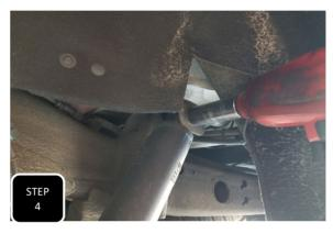
**Step 4** First, apply pressure to the diff with the adjustable jack. Next, to access the upper shock mount more easily, cut a slit in the wheel well liner and remove the upper mounting bolt of the shock.
