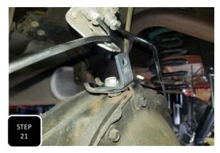
**Step 21** Remove the "O" ring that is on the factory mounting bolt for the brake line bracket at the top of the diff. Next, attach the provided brake line bracket to the top of the diff using this bolt and tighten.
