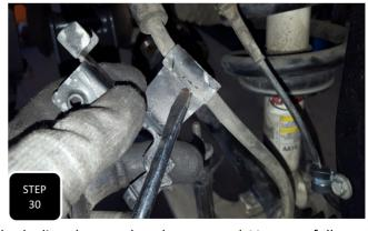
**Step 30** There is a mounting bracket on the middle of the soft brake line that needs to be removed. Very carefully, cut a groove in bracket where it wraps around the line. This will create a weak spot so you can use a flat head screw driver to pry the bracket open and remove it. **NOTE: BE VERY CAREFUL NOT TO CUT ALL THE WAY THROUGH THE BRACKET OR**
