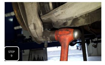
**Step 9** Loosen the lower ball joint nut, but do not remove. Next, hit the side of the spindle, right at the nut, with a hammer to break the ball joint loose. The nut will catch the spindle.
