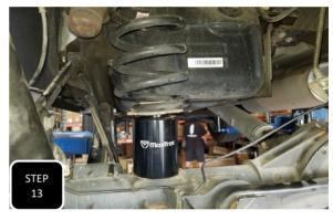
**Step 13** Locate the coil spacers and loosely install them along with the factory coils and isolators. Once both are in place, jack up the axle to apply pressure to the coils and assure that they are properly seated.
