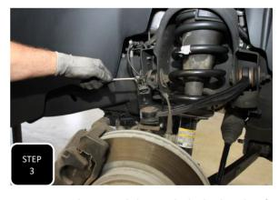
**Step 3** Separate the ABS line from the brake line bracket at the upper control arm and then unbolt the bracket from the control arm.
