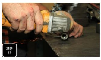
**Step 32** Remove the outer tie rod from the inner tie rod and mark a line 1/2" from the end of the threaded hole and cut this 1/2" section off. **NOTE: MAKE SURE YOUR CUT IS STRAIGHT SO THAT THE JAM NUT TIGHTENS UP PROPERLY.**
