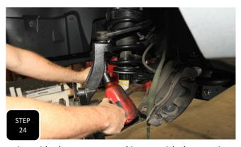
**Step 24** Install the steering knuckle assembly onto the the appropriate side that you are working on with the steering arm of the knuckle facing the front of the truck. Use the factory nuts at the upper and lower ball joints and tighten to factory specs. **NOTE: SLIDE THE AXLE INTO THE HUB BEFORE CONNECTING THE BALL JOINTS.**
