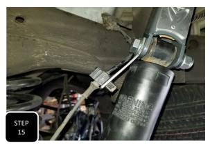
**Step 15** Loosely install the provided shock extenders with the logo facing outward, using the factory shock bolt. Next, attach the shock to the extender using the provided 14mm bolt, nut and washer and fully tighten both bolts. **NOTE: ON THE DRIVER'S SIDE, YOU WILL ATTACH THE PROVIDED ABS LINE BRACKET TO THE SHOCK MOUNTING BOLT AT THE FRONT OF THE EXTENDER WITH THE BRACKET POINTED STRAIGHT DOWN.**
