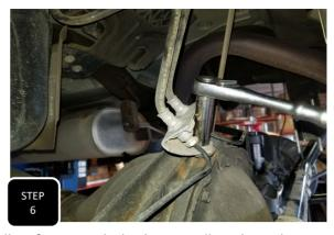
**Step 6** Unbolt the brakeline bracket from on top of the diff to allow for more slack when installing the coil spacers.
