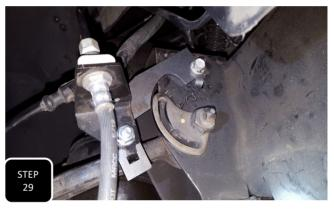
**Step 29** Locate the new brakeline mounting bracket and attach it to the side of the coil bucket using the factory brakeline bracket mounting bolt. Next, attach the factory brakeline bracket to the new brakeline bracket using the provided 8mm bolt, nut, and washers.
