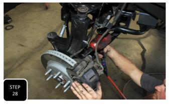
**Step 28** Unbolt the factory bracket that attaches the brakeline to the frame to gain extra slack in the line. Next, attach the brake caliper to the steering knuckle using the factory bolts and tighten.
