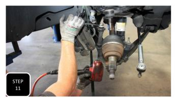
**Step 11** Unbolt the sway bar end link and remove.
