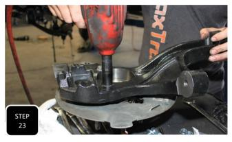
**Step 23** Place the factory hub assembly along with the factory dust shield onto the new steering knuckle and then flip the assembly over and attach the two together using the factory bolts and tighten.
