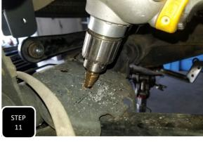
**Step 11** Locate the bump stop striker pads on the axle, then measure and mark an "X" 2 1/8" straight forward from the existing hole in the plate. Next, drill a 1/2" hole through your mark. **NOTE: CHECK THE FACTORY HOLE FOR WELD SLAG. IT MAY NEED TO BE CLEANED OUT TO ACCEPT A BOLT.**
