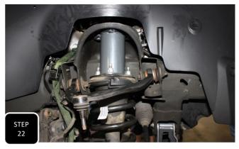
Step 22 Fully tighten the upper mounting nuts and the lower mounting bolts for both struts.
