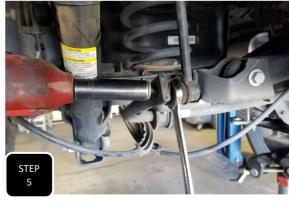
**Step 5** Unbolt both sway bar end links at both ends and remove.
