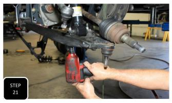
**Step 21** Loosely attach both lower control arms using the provided 5/8" hardware and then swing the arms up and loosely attach them to the bottom of the strut using the factory hardware. **NOTE: DO NOT FULLY TIGHTEN THE LOWER CONTROL ARM BUSHINGS UNTIL THE TRUCK IS BACK ON THE GROUND AT RIDE HEIGHT.**
