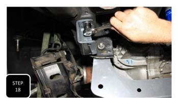
**Step 18** Install the sway bar drop down brackets using the supplied M10 bolts and washers. The open end of the bracket will face the inside of the truck and the bracket needs to swoop towards the rear of the truck.
