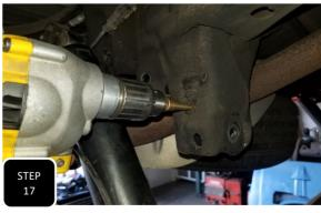
**Step 17** Using a scribe, trace the upper, side hole of the trac bar bracket, then remove the bracket and drill a 1/2" hole through your circle.
