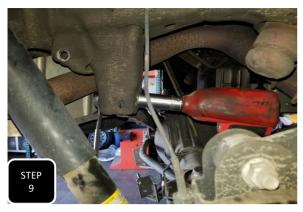
**Step 9** Unbolt the trac bar from the mount on the frame and separate.
