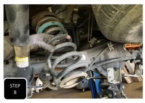
**Step 8** Lower down the axle and remove both coil springs. **NOTE: MAKE SURE TO SAVE THE RUBBER ISOLATORS FOR RE-INSTALLATION.**
