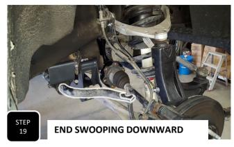
**Step 19** The ends of the sway bar originally swooped upward. The sway bar will now get re-installed with the ends swooping downward, the opposite of how they were. Use the factory bolts along with the provided nuts and washers to attach the sway bar to the drop down brackets and tighten.
