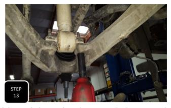
**Step 13** Remove the 3 nuts attaching the strut to the frame and the two bolts attaching the strut to the lower control arm, then remove the strut.
