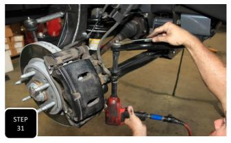
Step 31 Assemble the sway bar end links onto the truck and then tighten them up until the nut bottoms out.
