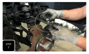
**Step 7** Separate the clip attaching the ABS line to the bracket you just removed from the top of the spindle and then open the clip and separate the ABS line from the clip.
