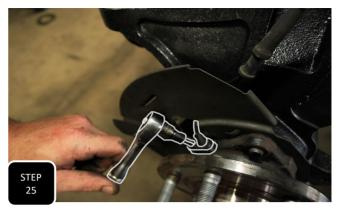
**Step 25** Unclip the ABS line from the frame, right next to where the brake line goes from soft to hard line. Next, use the extra slack gained to guide the ABS sensor down the steering knuckle and attach it to the wheel bearing using the factory bolt.
