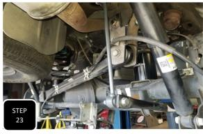
**Step 23** Install the new, longer sway bar end links using the factory bolt at the frame and the provided 12mm bolt at the sway bar, then tighten.
