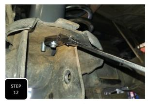
**Step 12** Install the provided bump stop extension and secure it by installing the provided 7/16" nut and washer on the most forward bolt and tighten. The further back bolt is just a guide. **NOTE: THIS AREA IS ONLY ACCESSABLE WHILE THE LOWER CONTROL ARM IS REMOVED FROM THE BRACKET ON THE AXLE.**
