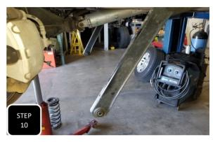
**Step 10** Make sure the adjustable jack under the diff has a provision to keep the diff from rotating, then unbolt both lower link arms from the axle, loosen the bolts at the frame, and allow them to both drop down, away from the axle. **NOTE: IF THE PINION IS NOT SUPPORTED, THE DIFF WILL WANT TO ROTATE DOWN.**
