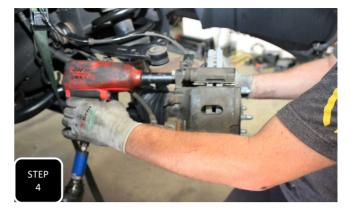
**Step 4** Unbolt the brake caliper and support it, up out of the way. **NOTE: NEVER ALLOW THE BRAKE CALIPER TO HANG BY THE BRAKE LINE.**
