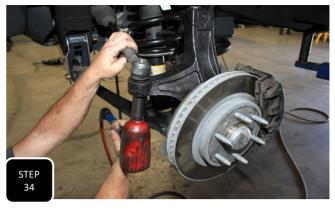
**Step 34** Once both ends are trimmed down, thread them back together and attach the tie rod to the steering knuckle using the factory nut.
