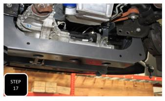
**Step 17** Loosely install the rear subframe using the factory hardware. The notch in the vertical rise of the subframe goes on the driver's side, facing forward to allow for clearance with the diff.
