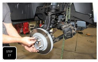
**Step 27** Install the rotor and secure the factory retainer screw.
