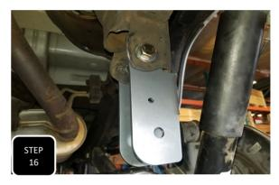
**Step 16** Loosely install the provided trac bar bracket onto the factory trac bar bracket on the passenger side frame using the provided 14mm bolt and zinc plated crush tube. The rearward facing ear of the provided bracket will install "**inside**" the factory bracket and the forward facing ear will install on the "outside" of the factory bracket.
