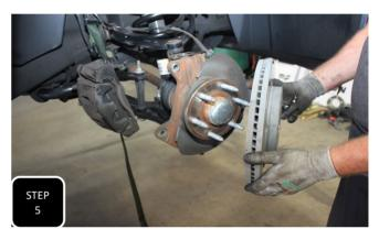
Step 5 Unbolt the rotor retainer bolt and then remove the rotor. NOTE: THE ROTOR SHOULD JUST POP OFF. IF IT DOES NOT JUST POP OFF, YOU WILL NEED TO HIT THE WHEEL MOUNTING SURFACE OF THE ROTOR WITH A HAMMER UNTIL THE RUSTY BOND IS BROKEN AND THE ROTOR POPS OFF.
