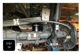
**Step 19** Loosely attach the trac bar to the new drop down bracket using the factory bolt and nut. **NOTE: DO NOT FULLY TIGHTEN THIS BOLT UNTIL THE TRUCK IS BACK ON THE GROUND AT RIDE HEIGHT.**
