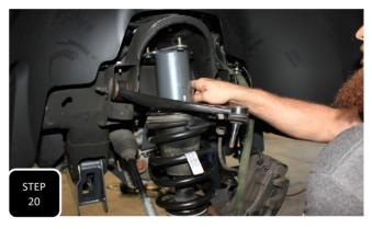
**Step 20** Locate the two struts and attach the strut spacer to the top using the factory nuts. Next, loosely install both sides using the provided nuts. **NOTE: THE SPACERS WILL ONLY FIT ONE WAY AND DO NOT FULLY TIGHTEN THE NUTS AT THE FRAME AT THIS TIME.**
