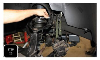
**Step 26** Using the provided loom clamps and factory 6 mm bolts, guide and attach the ABS line up the back side of the neck of the steering knuckle and to the upper control arm.
