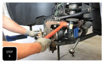
**Step 8** Loosen the upper ball joint nut, but do not remove. Hit the side of the spindle, right at the ball joint, with a hammer to break the ball joint loose. The nut will catch the spindle.
