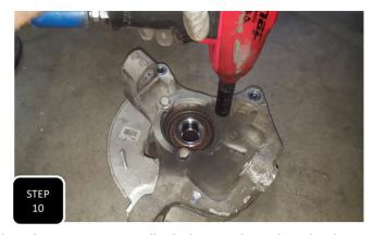
**Step 10** Remove the spindle and set it face down on the wheel studs. Next, remove all 3 bolts attaching the wheel bearing to the spindle and separate the two.
