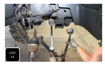
**Step 14** Unbolt both lower control arm mounting bolts and remove the lower control arm.
