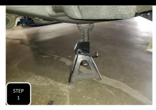
**Step 1** Jack up the rear of the truck and support under the frame rails with jack stands. Keep an adjustable jack under the diff for height adjustment.
