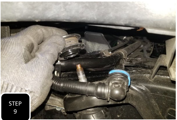
Step 9 Lower the truck back to the ground and re-attach the shocks. NOTE: THE REAR COILS ARE VERY TOUGH TO COMPRESS AND WILL LIFT THE TRUCK OFF OF THE CAR LIFT. LOWERING THE TRUCK TO THE GROUND ALLOWS THE WEIGHT OF THE TRUCK TO COMPRESS THE SPRINGS.
