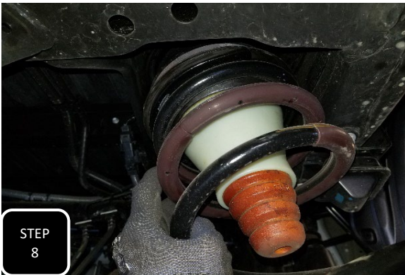
Step 8 Re-install the springs back into the truck and make sure the bottom of the coil indexes properly on the coil seat.
