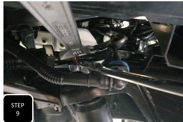
Step 9 Lower the truck back to the ground and re-attach the shocks. NOTE: THE REAR COILS ARE VERY TOUGH TO COMPRESS AND WILL LIFT THE TRUCK OFF OF THE CAR LIFT. LOWERING THE TRUCK TO THE GROUND ALLOWS THE WEIGHT OF THE TRUCK TO COMPRESS THE SPRINGS.
