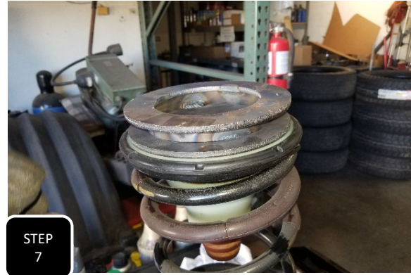
Step 7 Install the spacer on top of the coil with the centering nipple inside of the bump stop housing.
