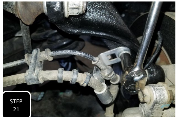
Step 21 Attach the brake/ABS line guide bracket to the side of the spindle using the factory bolt and tighten.
