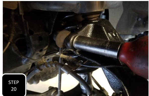
Step 20 Attach the sway bar end link to the spindle using the factory nut and tighten.
