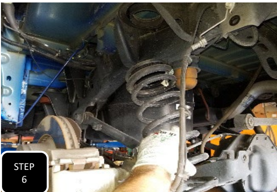
Step 6 Lower the axle and remove both rear coils.
