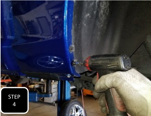
Step 4 Remove the plastic wheel liner on both sides to gain access to the upper shock mount.
