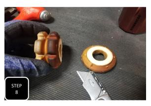
Step 8 Locate the factory bump stop and cut one rib off of the end of it.
