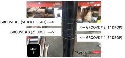
**Step 6** Locate your new struts and set the ring to the proper groove according to the picture above. Make sure the snap ring fully engages into the groove.
