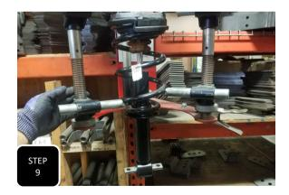
**Step 9** Slide the new coil seat onto the strut, then install the strut up through the bottom of the coil. **NOTE: MAKE SURE TO INSTALL THE BUMP STOP UP INTO THE CUP ON THE BOTTOM OF THE STRUT TOP BEFORE INSTALLING THE STRUT.**
