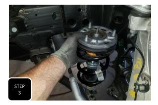
**Step 3** Unbolt both of the bolts attaching the lower control arm cross brace to the lower control arm and remove. Next, remove the strut assembly through the opening in the lower control arm.
