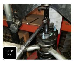
**Step 11** Install the factory strut top on the new strut using the provided M14 nut and tighten down. **NOTE: MAKE SURE THE TOP IS CLOCKED PROPERLY WITH THE LOWER STRUT MOUNT.**
