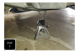
**Step 1** Jack up the front of the vehicle and support under the frame using jack stands.
