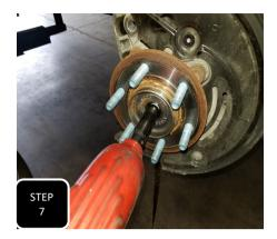
**Step 7** For 4wd models, remove the dust cap at the middle of the wheel bearing and then remove the axle retaining nut.
