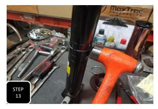
**Step 13** Install the snap ring retainer over the clip. If it does not slide over the clip, use a hammer to tap the clip into the groove until it fully seats. **NOTE: THE RETAINER MUST GO COMPLETELY OVER THE SNAP RING AND SEAT OR YOUR SUSPENSION COULD FAIL.**
