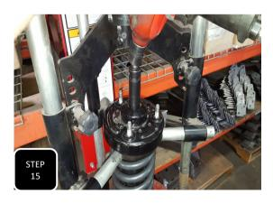
**Step 15** Insert the new strut into the coil and attach it to the factory strut top using the provided M14 nut. **NOTE:** MAKE SURE TO PROPERLY ALIGN THE TOP WITH THE BOTTOM.
