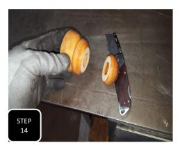
**Step 14** Install the supplied lower coil seat then cut down the factory bump stop by one rib and slide the bump stop onto the shock shaft.
