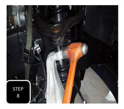
**Step 8** Loosen the upper ball joint then hit the side of the spindle with a hammer to break the ball joint loose. The nut will catch the spindle, then separate. **NOTE: NEVER HIT THE BALL JOINT ON THE THREADS.**
