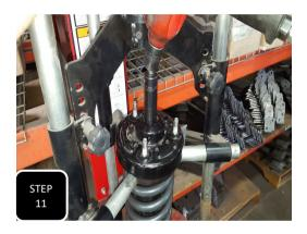
**Step 11** Place the strut assembly into a strut compressor to safely compress the coil, then remove the retaining nut and then the strut. **NOTE: TAKE NOTE OF THE POSITION OF THE STRUT TOP AND BOTTOM IN RELATIONSHIP TO EACH OTHER.**
