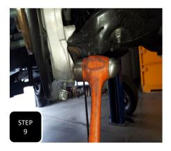
**Step 9** Loosen the lower ball joint then hit the side of the spindle with a hammer to break the ball joint loose. The nut will catch the spindle, then separate. **NOTE: NEVER HIT THE BALL JOINT ON THE THREADS.**
