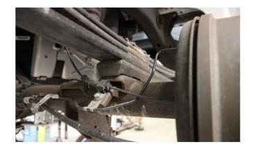
Step 6 With the axle supported, remove the U-bolts and spring plates on one side only.
