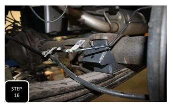
**Step 16** Once the axle is above the leaf spring on both sides and the leaf springs are both loosely installed, line up the provided axle relocators with the center pin on the spring and the attached brake line bracket facing the rear of the truck. Next, lower the axle into the relocators and assure the ears fit all the way up into the underside of the spring perch.
