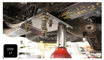
**Step 17** Place the provided U-bolt retainer plates on top of the factory spring perch with the bent ears facing in the direction of the front and back of the truck and then loosely install the factory U-bolts facing downward and through the provided spring plate under the leaf spring. Next, torque the U-bolts to 90 ft/lbs.
