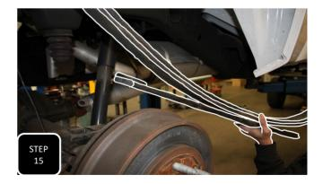
**Step 15** Repeat steps 6-16 on the other side. **NOTE: BE CAUTIOUS NOT TO STRETCH ANY ABS LINES OR BRAKE LINES AND IF PIVOTING THE AXLE SIDE TO SIDE, MAKE SURE IT IS SECURELY ATTACHED TO THE JACK.**
