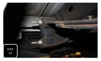
Step 14 Jack up the axle and loosely re-install the leaf spring under the axle using the factory bolts.
