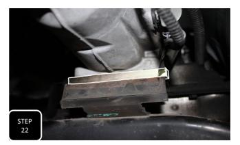
**Step 22** 2007-2013 models, install the gold, 1/2" tall transmission spacer between the trans and trans mount using the provided M10 bolts and washers. 2014-2018 models use the silver, 1/4" tall spacer. NOTE: IF DRIVE LINE VIBRATION IS EXPERIENCED, YOU CAN ALTERNATE OR STACK SPACERS. IF VIBRATION PERSISTS, IT IS RECOMMENDED TO TAKE YOUR TRUCK TO A DRIVE LINE SPECIALIST.
