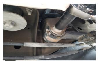
**Step 25** Once the wheels are back on and the truck is on the ground at ride height, jump on the rear bumper a few times to settle the suspension and then tighten all 6 leaf spring/shackle bolts. **NOTE: TIGHTENING THE LEAF SPRING/SHACKLE BOLTS WHILE THE TRUCK IS IN THE AIR CAN AFFECT THE RIDE HEIGHT, RIDE QUALITY, AND SHORTEN THE LIFE OF ALL OF THE BUSHINGS.**
