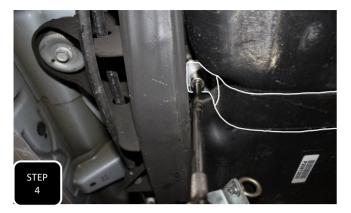
NOTE: AN ALTERNATE WAY OF GETTING THE AXLE ON TOP OF THE LEAF SPRINGS WITHOUT REMOVING THE GAS TANK WOULD BE TO BALANCE THE REAR END ON A JACK AND MOVE IT TO ONE SIDE WHILE YOU PIVOT THE SPRING DOWN. NEXT, JACK UP THE AXLE, RE-ATTACH THE SPRING AT THE SHACKLE SIDE, AND THEN MOVE THE AXLE OVER TO THE OTHER SIDE AND FOLLOW THE SAME STEPS WITH THE OTHER SPRING.
