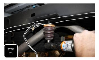
**Step 20** After cleaning up the sharp edges and spray painting the cut area for rust prevention, jack up the axle and mark where the axle will come into contact with the frame. Mark the center of the frame and then drill a hole using a 3/16" drill bit. Next, using the provided 1/4" self tapping bolt, attach the factory bump stop to the frame. **NOTE: THE FACTORY BUMP STOP CAN BE CUT DOWN TO ALLOW FOR MORE FREE TRAVEL.**
