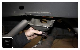
**Step 19** The factory bump stop extension bracket will need to be cut off the frame, so using a suitable cutting device, cut accross the outer mounting surface, inner mounting surface, and across the two bottom edges. Next, hit the bracket with a hammer and it should pop off. **NOTE: CONTROL THE DEPTH OF YOUR CUT SO THAT YOU DO NOT CUT THROUGH**
