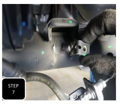
**Step 7** Using a suitable cutting devise, cut the brake line mounting bracket off of the axle and remove. **NOTE: THIS BRAKE LINE MOUNTING BRACKET IS LOCATED UNDER EACH SPRING PERCH, ON THE BACK SIDE OF THE AXLE TUBE AND WILL BE REPLACED BY ONE ATTACHED TO THE PROVIDED AXLE RELOCATOR.**
