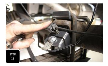
**Step 18** Attach the brake line guide bracket to the axle relocator using the provided M8 bolt, washer, and nut. Next, attach the ABS guide clip by pressing it into the slotted hole.
