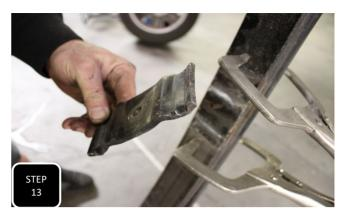
**Step 13** Install a couple clamps onto the leaf spring and remove the center pin. Next, remove and discard the U-bolt retainer plate and then re-install the center pin with the head on top of the leaf spring and the nut on the bottom. **NOTE: THIS IS OPPOSITE FROM THE WAY IT WAS ORIGINALLY INSTALLED.**
