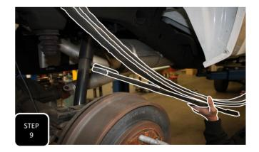
**Step 9** Unbolt the shackle mounting bolt and remove the front leaf spring bolt that you previously re-installed from the outside in, and then remove the leaf spring.
