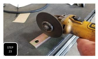
**Step 23** If drive line vibration is experienced on 4wd models, you will need to cut the provided spacer in half so that it will fit the bolt pattern of your T-case. It is recommended to start with the gold spacer. **NOTE: IF VIBRATION PERSISTS AFTER INSTALLING THE SPACER, IT IS RECOMMENDED TO TAKE YOUR TRUCK TO A DRIVE LINE SPECIALIST.**
