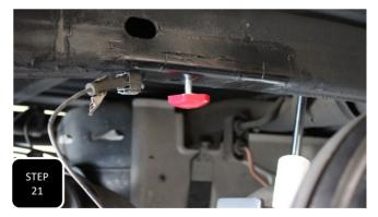
**Step 21** You also have the option of using the provided, low profile bump stop. If you choose to use this, then you will need to drill a 5/16" hole on your center mark and then tap that hole with a 3/8-16 tap. Next, thread the provided bump stop all the way up and hand tighten.
