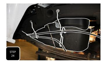
**Step 24** If you removed the gas tank to access the front leaf spring bolt, you will want to fully secure it now. Re-attach any wires that were disconnected and re-attach the filler neck. Lastly, re-install the factory plastic skid plate.
