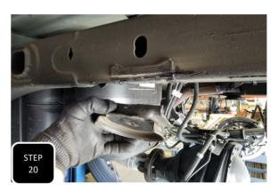
**Step 20** Once both cuts are made, it may help to hit the cut piece with a hammer until it breaks loose and then remove it from the frame. Next, clean up any sharp edges and spray paint for rust prevention.
