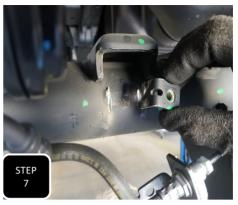
**Step 7** Using a suitable cutting devise, cut the brake line guide bracket off of the axle and remove.
