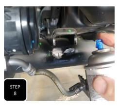
Step 8 Clean up any sharp edges and spray paint the area for rust prevention.
