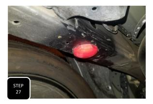
**Step 27** Insert the bump stop nut plates into the hole in the bottom of the frame that emerged after you removed the driver's and passenger's side factory bump stop plate. Thread the provided low profile bump stop into the nut plate until tight.
