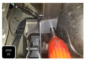
**Step 25** Loosely attach driver's side hanger support bracket using the provided M16 nut and washer at the hanger and the provided 1/2" bolt and washers at the frame. Tighten the 1/2" bolt at the frame, but do not fully tighten the 16mm spring bolt until the truck is on the ground at ride height.
