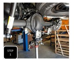
**Step 1** Jack up the rear of the vehicle and support under the frame rails with jack stands. Leave an adjustable jack under the differencial for height adjustment.
