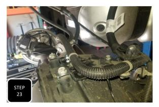
**Step 23** Locate the three "Z" shaped brake line brackets and loosely attach them to the factory bracket first using the provided hardware, and then to the diff using the factory hardware. The provided brackets are designed to push the factory bracket down and forward for more clearance between the diff and the bed.
