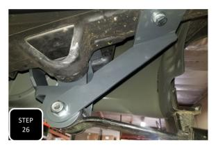
**Step 26** Insert the pass side, zinc plated nut plate into the hole in the outside of the frame, just back from the front leaf spring mount. **NOTE: THE NUT WILL LINE UP WITH THE SLOTTED HOLE IN THE BOTTOM OF THE FRAME.** Again, do not fully tighten the leaf spring bolt until the truck is on the ground at ride height.
