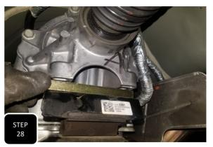
**Step 28** Remove both mounting bolts that attach the transmission to the mount at the cross member at the rear of the trans. Jack the trans up, insert the provided 1/2" tall, gold spacer, and tighten down using the factory bolts. **NOTE: THE USE OF THE PROVIDED 1/4"**, **SILVER SPACER MAY ONLY BE NEEDED IF DRIVE LINE VIBRATION IS EXPERIENCED.**
