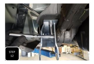
**Step 12** Locate the driver's side hanger and loosely install it into the driver's side, front leaf spring mount. Use the factory bolt at the main leaf spring hole and the provided 7/16" bolt, nut, and washer up through the top of the hanger. Tighten the 7/16" bolt first and then the main leaf spring bolt.
