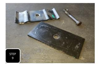
**Step 9** The leaf pack will now need to be dis-assembled. Attach two clamps to the spring and remove the center pin along with the U-bolt retainer plate and the factory 2 degree shim. (Only 2019 models have this shim) **NOTE: DISCARD THE U-BOLT RETAINER PLATE. IT DOES NOT GET RE-USED.**
