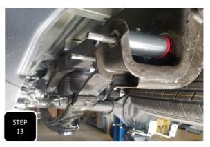
**Step 13** Jack up the axle and loosely re-install the leaf spring underneath the axle using the provided 16mm bolt at the front of the spring and the factory bolt at the shackle.
