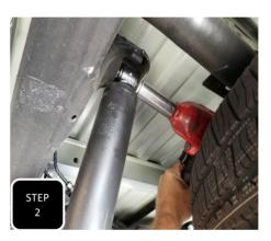
**Step 2** Jack up the adjustable jack slightly to apply pressure to the axle then unbolt both shocks at both ends and remove.
