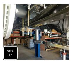
Step 17 Repeat steps 3-13 on the other side then when both sides are complete, torque the U-bolts to 100 ft/lbs.
