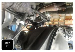
**Step 22** Unbolt the three bolts attaching the brake line bracket to the top of the differencial then pull it slightly up and forward.
