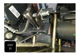
**Step 15** Locate the brake line mounting bracket still attached to the brake line and bend the guide tab to a flat position. Next, attach this bracket to the mounting bracket on the back side of the axle relocator using the provided M8 bolt, nut, and washer.
