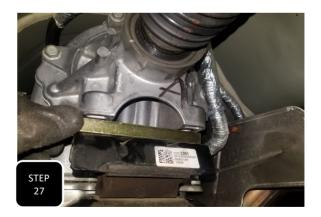
**Step 27** Remove both mounting bolts that attach the transmission to the mount at the cross member at the rear of the trans. Jack the trans up, insert the provided 1/2" tall, gold spacer, and tighten down using the factory bolts. **NOTE: THE USE OF THE PROVIDED 1/4", SILVER SPACER MAY ONLY BE NEEDED IF DRIVE LINE VIBRATION IS EXPERIENCED.**
