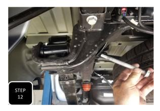
**Step 12** Jack up the axle and loosely re-install the leaf spring underneath the axle using the provided 16mm bolt at the front of the spring and the factory bolt at the shackle.
