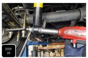
**Step 29** Install the wheels and tires then lower the truck to the ground. Jump on the rear bumper a few times then tighten up all 6 leaf spring/shackle bushings while the truck is at ride height.
