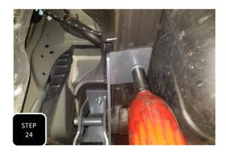
**Step 24** Loosely attach driver's side hanger support bracket using the provided M16 nut and washer at the hanger and the provided 1/2" bolt and washers at the frame. Tighten the 1/2" bolt at the frame, but do not fully tighten the 16mm spring bolt until the truck is on the ground at ride height.
