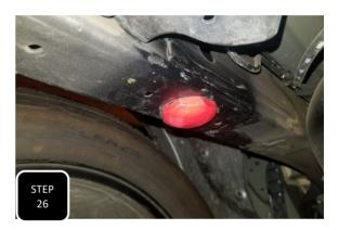
**Step 26** Insert the bump stop nut plates into the hole in the bottom of the frame that emerged after you removed the driver's and passenger's side factory bump stop plate. Thread the provided low profile bump stop into the nut plate until tight.
