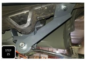
**Step 25** Insert the pass side, zinc plated nut plate into the hole in the outside of the frame, just back from the front leaf spring mount. **NOTE: THE NUT WILL LINE UP WITH THE SLOTTED HOLE IN THE BOTTOM OF THE FRAME.** Again, do not fully tighten the leaf spring bolt until the truck is on the ground at ride height.
