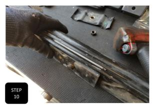
**Step 10** Slide the center pin through the factory 2 degree shim and install the pin down through the top of the leaf spring with the thick end of the shim facing the front of the truck. Then tighten the center pin. **NOTE: ONLY 2019 MODELS HAVE THIS 2 DEGREE SHIM.**
