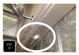
**Step 23** Insert the driver's side, zinc plated nut plate into the hole in the outside of the frame, just back from the front leaf spring mount. **NOTE: THE NUT WILL LINE UP WITH THE SLOTTED HOLE IN THE BOTTOM OF THE FRAME.**
