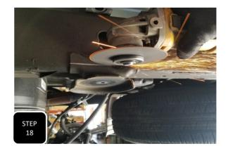
**Step 18** Unbolt the brake line guide bracket on the inside of the driver's side frame rail and support out of the way. Next, you will need to cut off the welded on bump stop plate using a suitable cutting device. Make a clean cut on each side of the frame rail.
