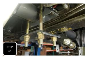
**Step 14** Place the U-bolt retainer plate on top of the original spring plate and run the new U-bolts downward though the provided spring perch under the leaf pack and tighten. **NOTE: THE U-BOLTS WILL INSTALL JUST LIKE THE FACTORY ONES DID. DO NOT TORQUE THE U-BOLTS DOWN AT THIS TIME**
