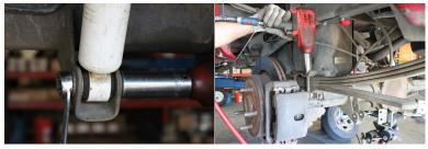
5) Unbolt the leaf spring at both ends along with the shackle and remove.
