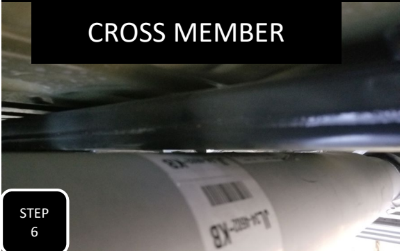
Step 6 Models with a 1 piece drive shaft have a cross member and a bed rib, both located closer to the transmission, that the drive shaft will slightly contact when the suspension bottoms out.
