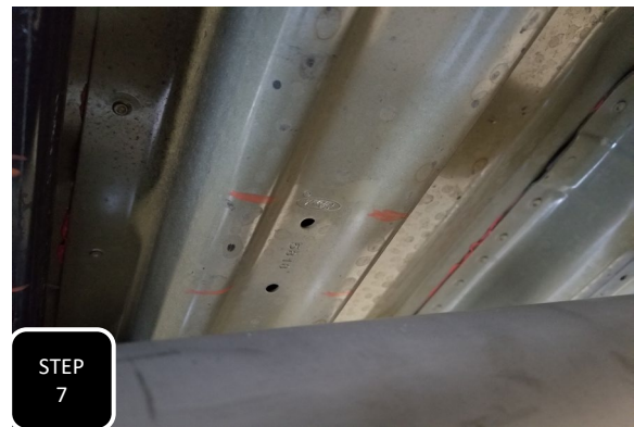
Step 7 With the axle jacked up and the drive shaft close to where it will contact, mark a center line for where the drive shaft is going to contact both the crossmember and the bed rib. Next, mark about 2 inches out both ways from your center line. This will be the area that you are going to clearance to avoid contact.
