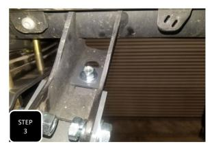
**Step 3** Slide the extender over the factory shock mount on the axle and loosely install the hardware. Install the flat washers onto the 1/2" bolts, install the 1/2" bolts through the factory shock hole, from the outside facing inward, then attach the 1/2" lock washer and jam nut. Then place the square plate over the ovalized opening inside the factory shock mount and attach it to the extender using the supplied 7/16" hardware.
