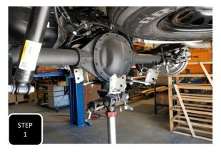
**Step 1** Jack up the rear of the truck and support under the frame rails with jack stands. Keep an adjustable jack under the axle for height adjustment.
