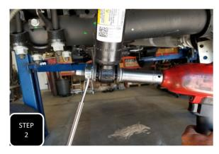
**Step 2** Unbolt both lower shocks from the axle and pivot them out of the way.
