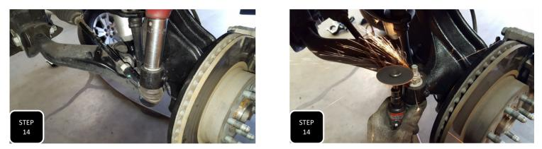
**Step 14** Re-attach the tie rod ,from the bottom up, using the factory nut and tighten to factory specs. Next, If you plan on running 17" wheels, using a suitable cutting devise, trim off the end of the tie rod shank where the non threaded part meets the threaded part. **NOTE: THIS WILL KEEP THE TIE ROD FROM HITTING THE WHEEL.**
