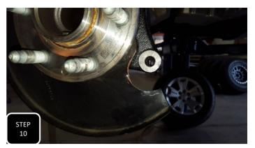
**Step 10** The dust shield will need to be trimmed to clear the brake caliper at the lower mounting hole. Mark a generous radius and trim this area using a suitable cutting device. Clean up any sharp edges and spray paint for rust prevention.
