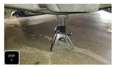
**Step 1** Jack up the front of the of the vehicle and support under the frame rails with jack stands. Remove both front tires and proceed with one side at a time.
