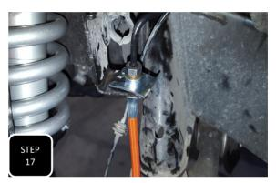
**Step 17** Re-attach the factory bracket at the frame using the factory bolt and then attach the brake line to the bracket using the new clip. Now you will need to bleed any and all air out of the braking system by opening up the bleeder screw on the brake caliper until only fluid comes out.
