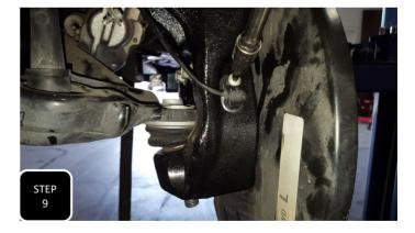
**Step 9** Unclip the ABS guide from the brake line bracket on the frame then remove the ABS guide clip near the upper control arm so that you can gain enough slack to attach the sensor to the spindle. **NOTE: CYCLE THE SPINDLE BACK AND FORTH IN ITS TURNING RADIUS TO ENSURE THE ABS LINE DOES NOT GET TIGHT.**
