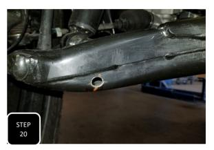
**Step 20** Drill a 1/2" hole where your two lines cross. Using a step bit will make the drilling much easier. **NOTE: THIS HOLE IS TO ALLOW FOR MORE CLEARANCE BETWEEN THE BANJO BOLT ON THE BRAKE CALIPER AND THE CONTROL ARM WITHOUT SACRIFICING TURN RADIUS.**
