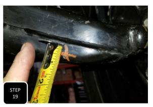
**Step 19** For 2020 and newer models, measure and mark a line 3 1/4" over from the center of the steering stop and another 1/2" down from the weld on the lower control arm.
