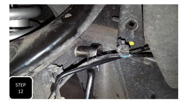
**Step 12** You will need to remove the clip that attaches the brake line to the bracket at the frame and pull the hard line through to gain enough slack to attach the brake caliper to the spindle. Next, unbolt the bracket from the frame, just under the upper control arm.
