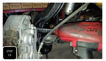
**Step 13** Attach the brake caliper to the spindle using the factory bolts and tighten to factory specs.
