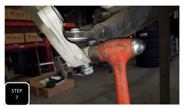
**Step 7** Loosen the upper and lower ball joint nuts, but do not remove them. Hit the side of the spindle (right at each ball joint) with a hammer to break the ball joint loose. The nut will catch the spindle, then remove the spindle. **NOTE: NEVER HIT THE BALL JOINT ON THE THREADS.**
