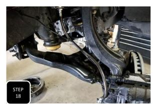
Step 18 Attach the ABS line to the brake line using 2 of the supplied 5" zip ties.
