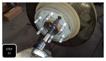
Step 11 Install the brake rotor and secure by snugging down the factory retainer bolt.
