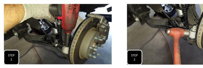
**Step 2** Remove the nut attaching the outer tie rod to the steering knuckle and then break loose by hitting the side of the spindle with a hammer right at the joint. **NOTE: NEVER HIT THE TIE ROD ON THE THREADS**
