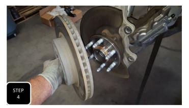
Step 4 Unbolt the rotor retainer screw and remove the brake rotor.
