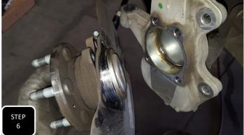
**Step 6** Unbolt all 4 wheel bearing bolts and remove the wheel bearing. **NOTE: MAKE SURE TO RETAIN THE FACTORY BACKING PLATE. IT WILL GET RE-INSTALLED.**
