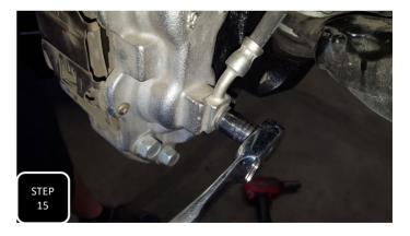
**Step 15** Unbolt the factory brake line at the frame and at the caliper and remove. Next, attach the new brake line at the frame first and allow brake fluid to run through before attaching to the caliper. **NOTE: ALLOWING FLUID TO RUN THROUGH THE NEW LINE WILL SPEED UP THE BLEEDING PROCESS.**
