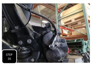
**Step 16** When attaching the banjo end of the brake line to the brake caliper, 2020+ models will use the new, thin head banjo bolt with one new copper washer on each side of the banjo and attach the line with the banjo fitting angled towards the brake caliper and up/outward like shown in the second picture. 2015-2019 models will use the factory banjo bolt.
