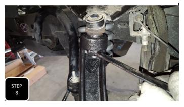
Step 8 Install the new spindle using the factory nuts and torque to factory specs.
