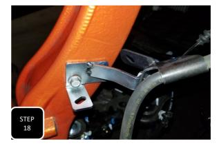
**Step 18 (Driver's Side)** Locate the provided D120 bracket. Attach the factory brake line bracket to it using the provided M6 bolt, nut, and washer. Next, attach the bracket to the spindle using a factory M6 bolt and tighten both.
