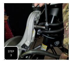
**Step 3** Unbolt both the brake line bracket and the ABS line bracket from the neck of the spindle and separate. Save the bolts for use during installation.
