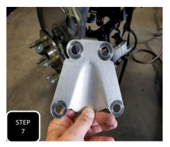
**Step 7** Remove the wheel bearing by unbolting all four mounting bolts and set the bearing off to the side. The retainer plate from the back side can be disgarded.
