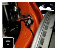
Step 16 Attach the ABS sensor and the guide bracket just above it using factory M6 bolts and tighten.
