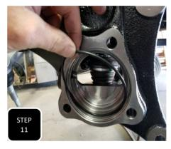
**Step 11** Using a dental pic or a small screw driver, remove the "O" ring from the hub bore in the factory spindle and reinstall it into the hub bore of the new spindle.
