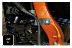
**Step 23 (Passenger Side)** For 2020+ models. Locate the P120 bracket and attach the factory brake line bracket to it using the provided M6 bolt, nut, and washer. Next, attach the bracket to the spindle using a factory M6 bolt.
