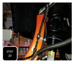
**Step 20 (Driver's Side)** Neately guide the ABS & brake pad sensor wires up the neck of the spindle and attach them to the upper mounting hole using the provided 1/4" loom clamps and a factory M6 bolt.
