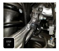
**Step 21 (Drivers Side)** Attach the 2 wires together at the rubber bushings using the provided zip ties. Next, attach the ABS wire to the upper control arm using the provided 3/8" loom clamp and factory M6 bolt.
