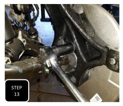
**Step 13** Install the wheel bearing along with the factory dust shield using the factory bolts and tighten.
