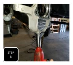
**Step 8** Loosen but do not remove the nuts for the upper and lower ball joints.
