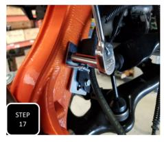
**Step 17 (Driver's Side)** For 2019 models, Locate the provided D1 bracket. For 2020+ models skip to step 18. Attach the factory brake line bracket to it using the provided M6 bolt, nut, and washer. Next, attach the bracket to the spindle using a factory M6 bolt and tighten both.
