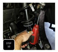
**Step 10** Attach the new spindle to the control arms using the factory nuts and tighten. **NOTE: IF YOU HAVE INSTALLED** A STRUT SPACER THEN THE USE OF A FLOOR JACK TO COMPRESS THE SUSPENSION WILL HELP IN ATTACHING THE SPINDLE.
