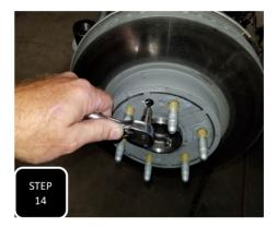
**Step 14** Slide the rotor onto the wheel studs and attach it to the hub using the factory retainer bolt.
