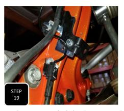
**Step 19 (Driver's Side)** Locate the provided bracket D2. Attach it to the mounting hole by the upper caliper bolt using a factory M6 bolt. Neatly guide the brake pad sensor wire and attach the two mounting clips to the ovalized holes in the D1 and D2 brackets.
