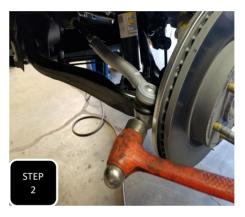
**Step 2** Remove the nut attaching the outer tie rod to the steering knuckle and then break loose by hitting the side of the spindle with a hammer right at the joint. **NOTE: NEVER HIT THE TIE ROD ON THE THREADS**
