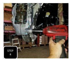
**Step 4** Unbolt both bolts attaching the brake caliper and support the brake caliper up out of the way. **NOTE: NEVER ALLOW THE BRAKE CALIPER TO HANG BY THE BRAKE LINE.**
