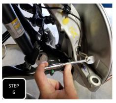
**Step 6** Unbolt the front side ABS wire bracket and the ABS sensor mounting bolt, then remove the sensor. Drape the sensor up out of the way so it does not get damaged during the install.
