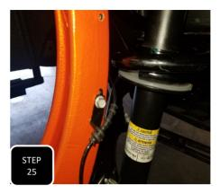
**Step 25 (Passenger Side)** Install the ABS sensor into the spindle using the factory bolt and tighten. Next, attach the two factory guide brackets to the neck of the spindle using a factory M6 bolt at each.
