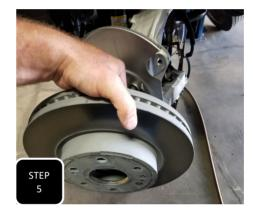
**Step 5** Unbolt the rotor retainer screw and remove the brake rotor.
