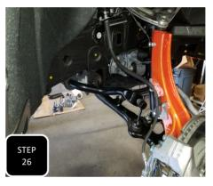
**Step 26 (Passenger Side)** Using the provided 1/4" loom clamp, attach the ABS wire to the top of the brake caliper side of the neck of the spindle using a factory M6 bolt.
