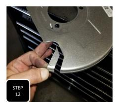
**Step 12** Locate the factory dust shield and mark a cut out about 1/2" down from the lower brake caliper ear opening. Using a suitable cutting device, cut out this marked section and clean up the edges.
