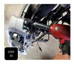
**Step 15** Install the brake caliper using the factory bolts and tighten.
