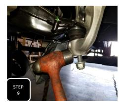
**Step 9** Break each ball joint loose by hitting the side of the spindle, right at the ball joint, with a hammer. The nut will catch the spindle, then remove both nuts and the spindle. **NOTE: NEVER HIT THE BALL JOINT ON THE THREADS.**
