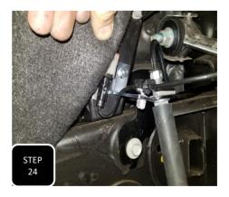
**Step 24 (Passenger Side)** Unhook the ABS guide clip from up near the hard brake line. Locate the P2 bracket and attach the bracket to the wheel well using the provided M6 bolt, nut, and washer. **NOTE: IT WILL HELP TO PULL BACK THE INNER FENDER A BIT AND INSTALL THE BOLT FROM THE BACK OF THE BRACKET.**
