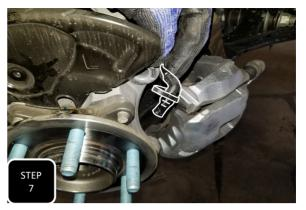
**Step 7** Unbolt the ABS sensor from the top of the hub, remove it, and then hang it up out of the way so that it does not get damaged during the install.
