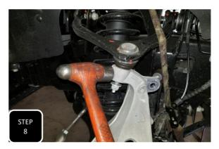
**Step 8** Loosen the nut at the upper ball joint, but do not fully remove it. Next, break the ball joint loose by hitting the side of the spindle, right at the ball joint, with a hammer. The nut will catch the spindle. **NOTE: NEVER HIT THE BALL JOINT ON THE THREADS.**
