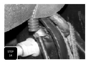
**Step 14** Remove the ABS guide clips at both the brake line bracket and at the side of the upper control arm mount, then cut off the plastic clip. This will allow for more slack in the line.
