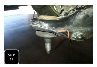
**Step 11** 2009-2014 models will require a good amount of trimming on the lower control arm. Using a suitable grinder, clearance about 1/4" off the bottom/front of the LCA and round off around the edges into the points where the control arm drops down. **NOTE: INSTEAD OF GRINDING, THE DUST CAP ON THE BACK OF THE WHEEL BEARING CAN BE REMOVED TO GAIN THE CLEARANCE NEEDED.**
