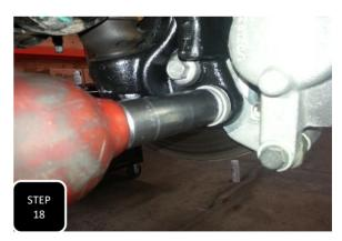
**Step 18** Remove the "U" shaped clip that secures the brake line to the bracket on the frame and pull the line downward to gain slack. Next, attach the brake caliper to the spindle using the factory bolts and tighten to factory specs.
