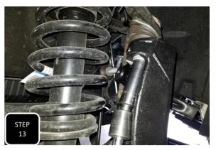
**Step 13** Install the new spindle using the factory ball joint nuts and tighten to factory specs. **NOTE: CYCLE THE SPINDLE BACK AND FORTH THROUGH ITS STEERING CYCLE TO ENSURE PROPER CLEARANCE OF THE LCA. IF THE LCA MAKES CONTACT, REMOVE THE SPINDLE AND CONTINUE CLEARANCING AS NEEDED.**
