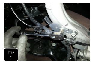
**Step 4** Unbolt the brake line guide bracket from the neck of the spindle then separate.
