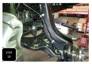
**Step 16** Use the supplied 1/4" and 3/8" adel clamps along with the supplied M6 bolts to guide the ABS wire safely up the neck of the spindle. The larger 3/8" clamp will be installed over a rubber sleeve on the wire. Cycle the spindle back and forth in its turn radius to ensure there is enough slack in the ABS wire.
