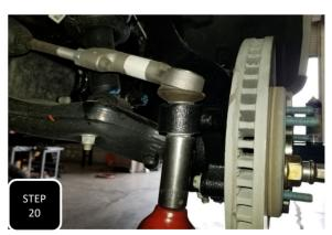
**Step 20** Re-attach the tie rod to the steering arm of the spindle using the facory nut and tighten. Next, repeat steps 1-20 on the other side.
