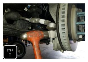
**Step 2** Unbolt the tie rod at the spindle and break it loose by hitting the side of the spindle, right at the joint, with a hammer and separate. **NOTE: NEVER HIT THE TIE ROD ON THE THREADS.**
