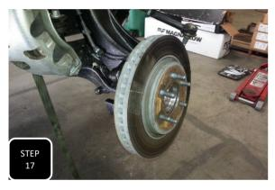
**Step 17** Install the brake rotor onto the wheel studs.
