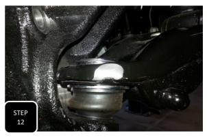
**Step 12** 2015-2020 models will require just a little bit of trimming on the front corner of the lower control arm. Using a suitable grinder, round off the corner of the LCA towards the front of the truck.
