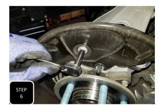
**Step 6** Remove the free floating brake rotor and then remove the upper mounting bolt on the dust shield behind it. **NOTE: IF THE BRAKE ROTOR DOES NOT JUST COME OFF, IT WILL HELP TO SPRAY WD-40 AROUND THE MIDDLE HOLE AND THEN HIT THE WHEEL MOUNTING SURFACE WITH A HAMMER TO JAR IT LOOSE.**
