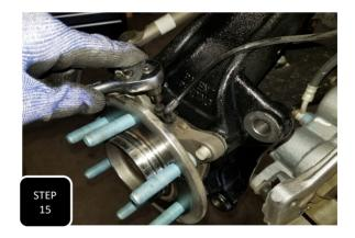
**Step 15** Attach the ABS sensor to the hub assembly using the factory socket head allen screw.
