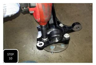
**Step 10** Remove the 4 wheel bearing bolts and then separate the wheel bearing from the factory spindle. Next, attach the wheel bearing to the new spindle using the factory bolts and tighten. **NOTE: THE FACTORY DUST SHIELD WILL NOT GET RE-USED.**
