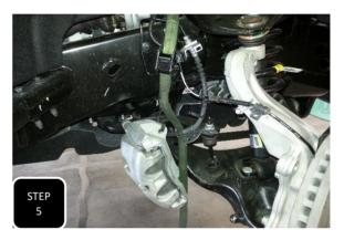
**Step 5** Unbolt both brake caliper bolts and support the brake caliper up out of the way. **NOTE: NEVER ALLOW THE BRAKE CALIPER TO HANG FROM THE BRAKE LINE.**
