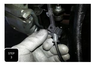
**Step 3** Unbolt the ABS line guide bracket from the neck of the spindle and then remove the plastic loom clamp from the line.
