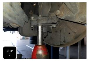
**Step 7** Use a floor jack under the lower control arm to compress the coil and then re-install the factory lower ball joint nuts and tighten to factory specs.
