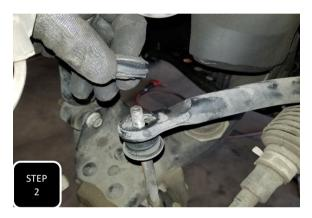
Step 2 Unbolt the sway bar end link from the sway bar and remove the upper bushing/washer.
