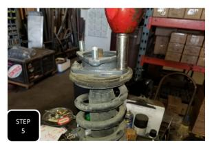
**Step 5** Remove the strut and attach the strut spacer to the top using the factory nuts, then tighten.
