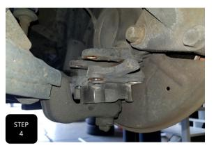
**Step 4** Unbolt the 4 bolts attaching the lower ball joint to the steering knuckle and allow it to separate.
