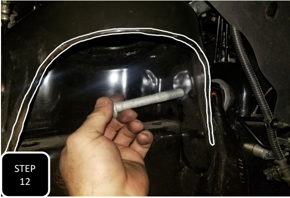
Step 12 Remove the bolts and the control arm.
