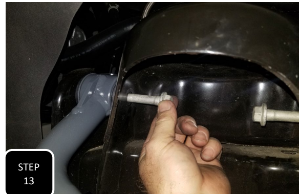
Step 13 Locate the new control arm with a ball joint that is off-set the same way as the control arm that you just removed and attach it to the frame using the factory bolts installed from the inside of the coil bucket outwards. NOTE: DO NOT FULLY TIGHTEN THESE BOLTS UNTIL THE VEHICLE IS ON THE GROUND AT RIDE HEIGHT.
