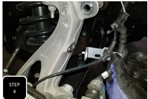
Step 4 Unbolt the brake line guide bracket from the neck of the spindle and separate.
