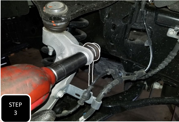
Step 3 Unbolt the sway bar end link from the neck of the spindle and separate.
