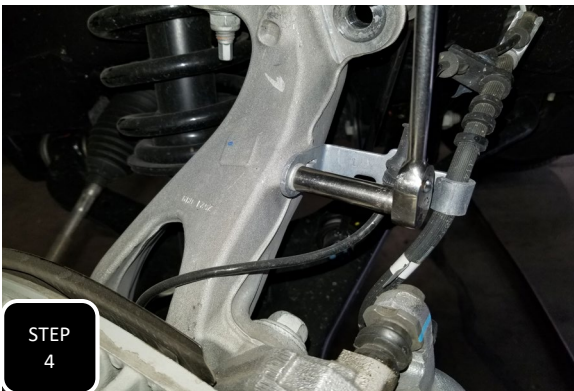
Step 4 Unbolt the brake line guide bracket from the neck of the spindle and separate.
