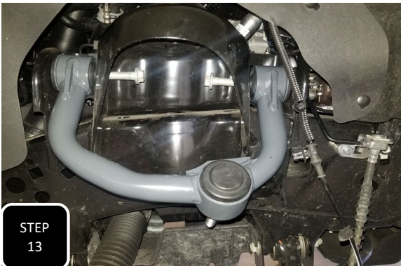
Step 13 Locate the new control arm with a ball joint that is off-set the same way as the control arm that you just removed and attach it to the frame using the factory bolts installed from the inside of the coil bucket outwards. NOTE: DO NOT FULLY TIGHTEN THESE BOLTS UNTIL THE VEHICLE IS ON THE GROUND AT RIDE HEIGHT.
