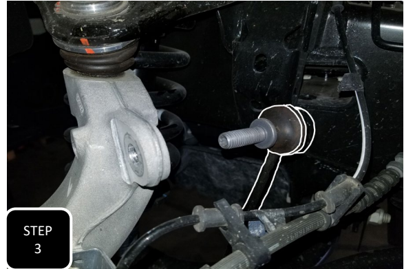
Step 3 Unbolt the sway bar end link from the neck of the spindle and separate.
