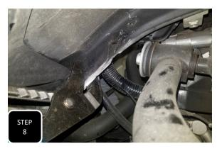
**Step 8** Using a large pair of pliars, bend the lip of the fender well outward to make room for the upper control arm mounting bolt to push out and past it. **NOTE: BE CAUTIOUS TO NOT PINCH OR DAMAGE ANY WIRING WHILE PERFORMING THIS STEP.**
