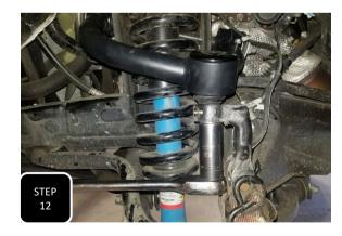
**Step 12** Connect the upper ball joint to the spindle and tighten to factory specs.
