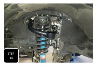
**Step 14** Re-attach the sway bar end link to the neck of the spindle and then re-attach both of the rubber skirts back into their original location.
