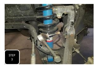
**Step 3** Unbolt the sway bar end link from the neck of the spindle and separate.
