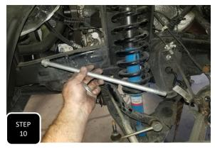
Step 10 Remove the long bolt that attaches the upper control arm to the frame and remove the control arm. NOTE: THIS WILL BE DIFFICULT TO REMOVE AS THE HEAD OF THE BOLT PASSES AND CONTACTS THE WHEEL WELL. USING A SCREW DRIVER ON THE BACK SIDE TO TAP IT THROUGH AND OR PLIARS TO GRAB AND SLIDE THE BOLT WILL BOTH HELP WITH THE REMOVAL.
