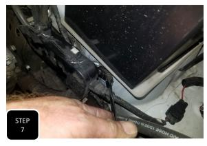
**Step 7** Unclip and or unbolt any wiring that is on the engine side of the fender lip near the front of the upper control arm so that it does not interfere with the removal of the upper control arm mounting bolt.
