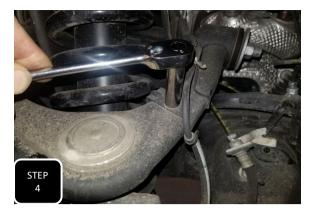
**Step 4** Open up the clamp attaching the ABS line to the upper control arm and then unbolt the bracket. This will allow for slack in the line while the spindle is separated from the upper control arm.
