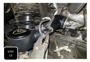
**Step 13** Attach the ABS guide bracket to the threaded post on the control arm using the provided nylock nut and then crimp the ABS line back into the guide clip.
