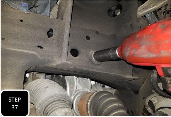
Step 37 Fully tighten both bolts on the driver's side diff drop bracket and torque to 85 ft/lbs.
