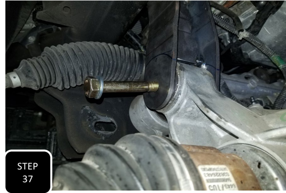
Step 37 Fully tighten both bolts on the driver's side diff drop bracket and torque to 85 ft/lbs.
