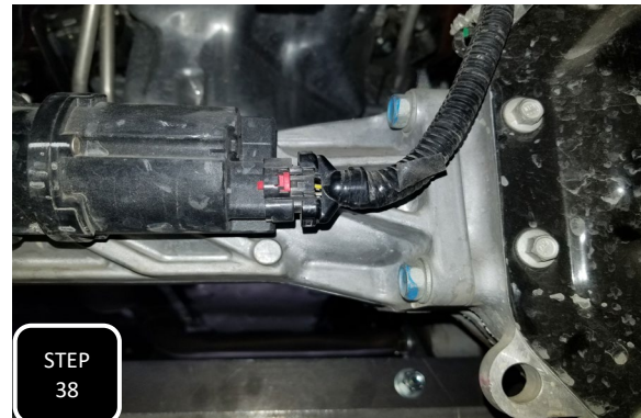
Step 38 There is a wire guide clip for the front diff electrical plug located on the frame near where the steering shaft meets the steering rack. This clip needs to be separated from the frame to allow for extra slack in the line. Next, Plug the pig tail into the diff and engage the red safety clip.
