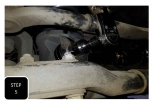
**Step 5** Lower the truck to the ground and drive forward and back about 10 feet to settle the suspension. Next, torque both trac bar mounting bolts to 250 ft/lbs.
