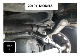
**Step 5** The steering wheel will now need to be straightened so start by breaking the two jam nuts on the tie rod loose. Next, turn the center collar until the wheel moves to straight. Drive the vehicle and then repeat steps if necessary and fully tighten the jam nuts when done.
