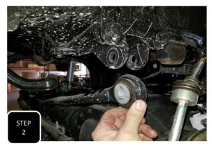
**Step 2** Remove the bolt attaching the trac bar to the bracket on the frame and separate. Allow the trac bar to rest on the axle.
