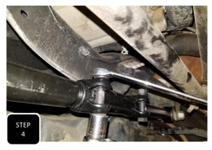
**Step 4** Adjust the collar on the trac bar in the direction needed until your measurements on both sides read the same. Then tighten down the clamps on the trac bar. **NOTE: MAKE SURE THE ADJUSTMENT CLAMPS ARE ORIENTED AWAY FROM THE AXLE AND FRAME.**
