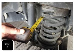
**Step 6** Find a consistant spot between the frame and the tire on both sides to take a measurement and compare to see which way the trac bar needs to be adjusted to center the axle to the frame.
