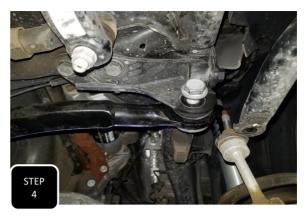
**Step 4** Loosely install the new adjustable trac bar using the factory hardware. The stamped arc in the trac bar needs to be towards the frame so that the trac bar clears the diff. Do not fully tighten the bolts yet. **NOTE: USE THE ADJUSTABILITY OF THE TRAC BAR FOR EASE OF INSTALLING THE BOLTS, BUT DON'T WORRY ABOUT FINAL**
