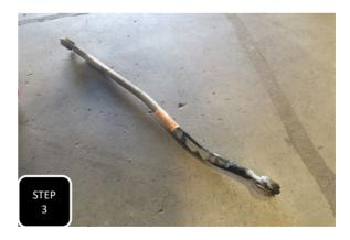
**Step 3** Unbolt the trac bar from the axle and completely remove the trac bar. Save the hardware for re-installation.
