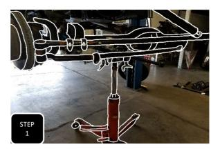
**Step 1** Jack up the front of the vehicle, place jack stands under the front axle, and remove both tires. **NOTE: REMOVING THE FRONT TIRES WILL ALLOW FOR ACCESS TO TRAC BAR MOUNTING POINTS.**
