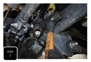
**Step 2** Unbolt the nut attaching the track bar to the axle and then brake the joint loose by hitting the side of the axle mount with a hammer. **NOTE: NEVER HIT THE ROD END ON THE THREADS.**
