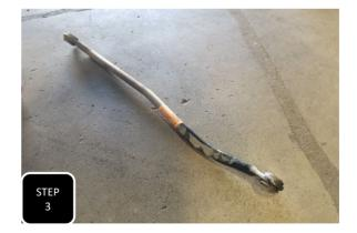
**Step 3** Loosen and remove the mounting bolt at the frame side of the trac bar and remove the factory trac bar.
