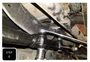
**Step 6** Adjust the collar on the trac bar in the direction needed until your measurements on both sides read the same. Then tighten down the clamps on the trac bar. **NOTE: MAKE SURE THE ADJUSTMENT CLAMPS ARE ORIENTED AWAY FROM THE AXLE AND FRAME.**
