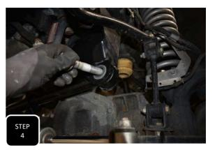
**Step 4** Loosely attach the new adjustable trac bar using the factory bolt at the frame and the provided nut at the axle then torque both to factory specs. The frame side bolt gets torqued to 406 ft/lbs and the axle side nut to 200 ft/lbs.
