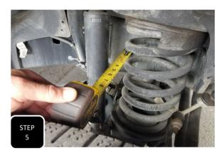
**Step 5** Find a consistant spot between the frame and the tire on both sides to take a measurement and compare to see which way the trac bar needs to be adjusted to center the axle to the frame.
