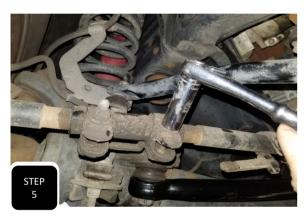
**Step 5** Loosen both of the clamps on the drag link adjuster and spin the collar until the steering wheel is straight and tighten both clamps back down. Next, go drive the truck to make sure the wheel is straight then make further adjustments as needed.
