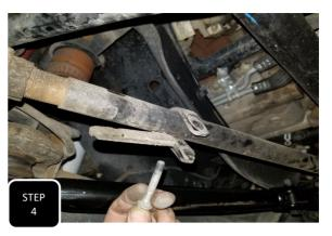
**Step 4** The steering wheel will now need to be straightened so start by unbolting and removing the safety tabe the for the drag link and sliding it out of the way.
