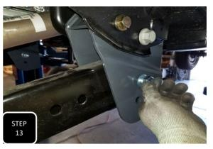
**Step 13** Swing the radius arm up and attach it to the new bracket using the provided M18 bolt. For a 4" lift attach the arm to the upper of the two holes and for a 6" or 8" lift attach it to the lower of the two holes.
