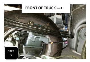
**Step 5** Working on one side at a time, remove the U-bolts and lower the axle down enough to remove the factory lift block and install the new, taller lift block. The block will need to be installed with the shorter side facing the front of the truck and with the bump stop stiker plate facing inward.
