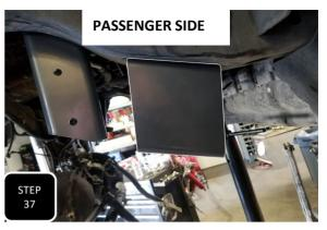
**Step 37** Intstall the new sway bar drop down brackets. You will notice that one of the vertical sides has more angle to it than the other. The more angled side will face the rear of the truck and open end of the bracket will face toward the middle of the truck. Attach each side to the frame using the factory nuts and tighten.
