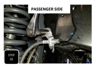
**Step 35** The passenger side ABS/ brake line bracket will mount the same as the driver's side and also require the unraveling of the factory hard brake line to line up with the new bracket.
