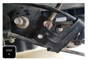
**Step 4** On the driver's side near the front spring hanger is a bolt on E-brake bracket. Unbolt this and install the provided extension bracket using the factory bolt at the frame and the provided M8 bolt, nut, and washers at the bracket.
