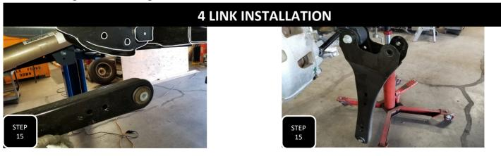
**Step 15** Loosen all 3 radius arm mounting bolts, 2 at the axle and 1 at the frame and then remove the radius arm. **NOTE: WORK ON ONE SIDE AT A TIME.**
