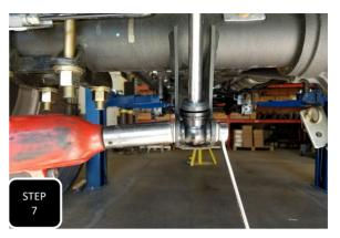
**Step 7** Install your new longer shocks using the factory hardware and tighten. **NOTE: MAX TRAC SHOCKS HAVE TO BE MOUNTED WITH THE BODY OF THE SHOCK AT THE AXLE AND THE SHAFT OF THE SHOCK AT THE FRAME. FOX SHOCKS WILL BE MOUNTED THE OPPOSITE OF THIS.**
