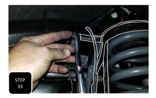
**Step 33** Separate both ABS line guide clips from the front of the coil bucket on the frame and install the new ABS/brake line bracket using the provided M8 bolts, nuts, and washers. **NOTE: THE DRIVER'S SIDE BRACKET IS THE LONGER OF THE TWO PROVIDED BRACKETS.**
