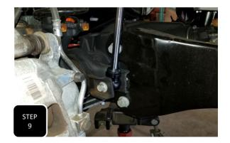
**Step 9** Loosely attach the new shock to hold the axle, then move the jack to the passenger side and repeat steps 6-9. **NOTE: THE SHOCKS WILL HOLD THE AXLE AS YOU MOVE THE JACK AND CONTINUE THROUGH THE INSTALL.**
