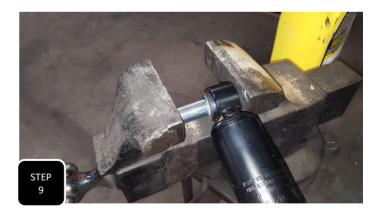
**Step 9** If installing Max Trac shocks, you will need to grease the bushings and use a bench vise to press in the shock sleeves.
