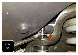
Step 32 Tighten up both ends of both front shocks.
