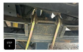
**Step 6** 2020+ dually models that do not have a factory lift block will need to remove the top side overload leaf spring and separation block. Next, the center pin of the leaf pack will need to be trimmed down and re-installed.
