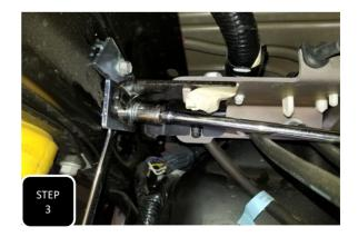
**Step 3** Unbolt the rear brake line guide bracket on the inside of the driver's side frame rail and install the provided drop down bracket using one of the factory bolts at the frame and the provided M8 bolt, nut, and washers at the bracket.
