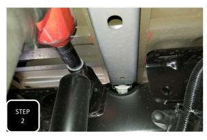
**Step 2** Unbolt both rear shocks at both ends and remove.
