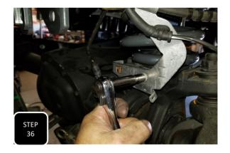
**Step 36** Using the factory bolt, re-attach the brake line bracket to the lower coil mount as it was originally.
