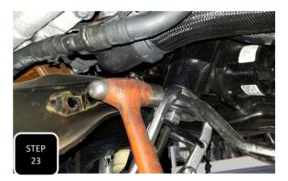
**Step 23** Using a 46mm socket, remove the pitman arm mounting nut. Next, apply tension to the arm using a pitman arm puller or a suitable 3 jaw puller. Hit the side of the pitman arm, right at the steering shaft, with a hammer a few times, very hard and then tighten down the puller some more. Proceed doing this until the pitman arm separates from the steering box. **NOTE: BE CAREFUL NOT TO DAMAGE THE STEERING BOX OR STEERING SHAFT.**
