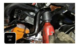
**Step 24** Apply a conservative amount of thread locker to the threads of the factory nut then attach the new drop down pitman arm to the steering box using the factory nut. Once tight, then torque to 350 ft/lbs. **NOTE: MAKE SURE TO INSTALL THE NEW PITMAN ARM IN THE EXACT SAME DIRECTION AS THE OLD ONE CAME OFF.**
