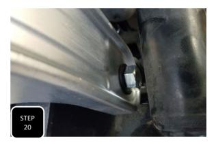
**Step 20** Insert the larger machined sleeves into the upper link arm hole at the axle side of the link. Both sleeves get installed from the outside facing inward then attach the link to the axle using the provided M18 bolt, nut and washers.
