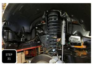
**Step 31** Move your adjustable jack under the driver's side of the axle and apply pressure so that you can remove the lower shock bolt and then lower the axle down. Next, Install the new lift coil with the factory rubber isolator on top, jack the axle back up and re-attach the shock. Repeat this step on the other side.
