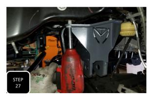
**Step 27** Locate the new trac bar bracket and attach it using the the factory nuts/3 bolt plate at the cross member and the factory 2 bolts under the frame then tighten.
