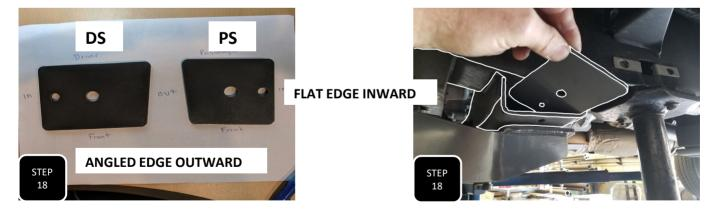
**Step 18** Locate the flat plate labeled DS and slide it into the cross member above the back of the 4 link bracket. Line up the hole and loosely attach the plate and bracket together using the provided M12-1.5 x 40 socket head allen bolt. **NOTE: THE DRIVER'S SIDE IS THE LONGER PLATE**
