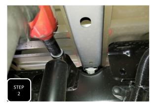
**Step 2** Unbolt both rear shocks at both ends and remove.
