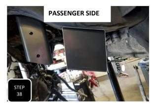
**Step 38** Intstall the new sway bar drop down brackets. You will notice that one of the vertical sides has more angle to it than the other. The more angled side will face the rear of the truck and open end of the bracket will face toward the middle of the truck. Attach each side to the frame using the factory nuts and tighten.
