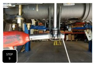
**Step 8** Install your new longer shocks using the factory hardware and tighten. **NOTE: MAX TRAC SHOCKS HAVE TO BE MOUNTED WITH THE BODY OF THE SHOCK AT THE AXLE AND THE SHAFT OF THE SHOCK AT THE FRAME. FOX SHOCKS WILL BE MOUNTED THE OPPOSITE OF THIS.**
