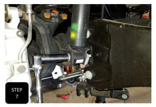
**Step 7** Move the adjustable jack to the driver's side and apply pressure to the axle. Next, unbolt the driver's side shock at both ends and remove.
