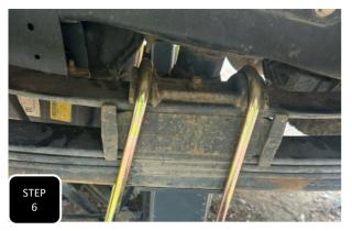
**Step 6** 2020+ dually models that do not have a factory lift block will need to remove the top side overload leaf spring and separation block. Next, the center pin of the leaf pack will need to be trimmed down and re-installed.
