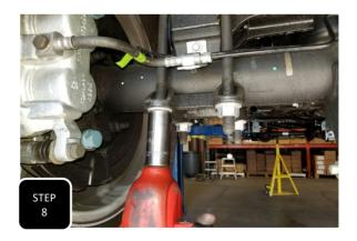
**Step 8** Once cut to length, install the U-bolts with the factory U-bolt plate and snug down. You will want to then loosen the U-bolts on the other side to allow the axle to rotate, and then fully tighten and torque the U-bolts to 140 ft/lbs. Next, install the block on the other side and torque down the U-bolts.
