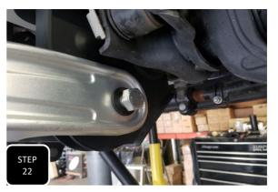
**Step 22** Remove the upper bolt attaching the radius arm on the other side so that the axle can be rotated. Next, insert two of the larger sleeves into the hole in the lower link and attach the lower link to the axle using the provided M18 bolt, nut, and washers. **NOTE: DO NOT FULLY TIGHTEN THESE BOLTS UNTIL THE TRUCK IS BACK ON THE GROUND AT RIDE HEIGHT.**
