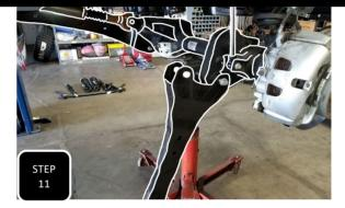
**Step 11** Loosen all 3 radius arm bolts, one side at a time. Then remove the upper bolt at the axle and the bolt at the frame and pivot the radius arm down out of the way. **NOTE: WORK ON ONE SIDE AT A TIME SO THAT THE AXLE IS SAFELY SUPPORTED AT ALL TIMES.**
