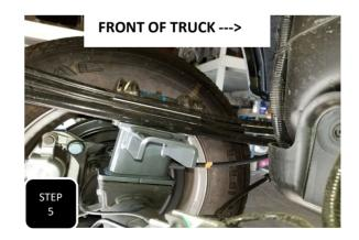
**Step 5** Working on one side at a time, remove the U-bolts and lower the axle down enough to remove the factory lift block and install the new, taller lift block. The block will need to be installed with the shorter side facing the front of the truck and with the bump stop stiker plate facing inward.
