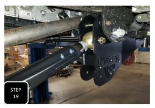
**Step 19** Locate 1 of the 4 arms. There should be 2 DS where the "MT" logo is facing up and the pinch bolts are facing outward. The PS arms are the opposite. Adjust the arm to a length of 32" from eye-eye with the grease fitting facing downward. Next, grease the rod end and loosely install it into the upper hole of the 4 link frame bracket using the provided 9/16" bolt, washers & nut. **NOTE: THE ROD ENDS ARE NOT PRE-GREASED AND REQUIRE GREASE FOR PROPER FUNCTION.**
