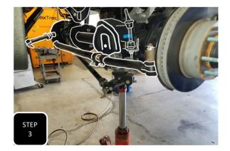
**Step 3** Unbolt the trac bar from the bracket on the frame and separate.
