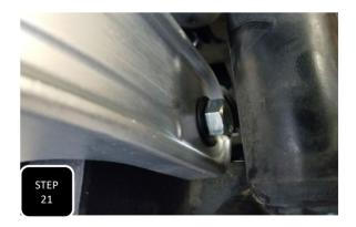
**Step 21** Insert the larger machined sleeves into the upper link arm hole at the axle side of the link. Both sleeves get installed from the outside facing inward then attach the link to the axle using the provided M18 bolt, nut and washers.
