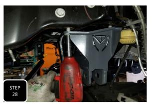
**Step 28** Locate the new trac bar bracket and attach it using the the factory nuts/3 bolt plate at the cross member and the factory 2 bolts under the frame then tighten. **NOTE: THE NEW TRAC BAR BRACKET WILL NOW LINE UP ON THE BACK SIDE OF THE ENGINE CROSS MEMBER.**
