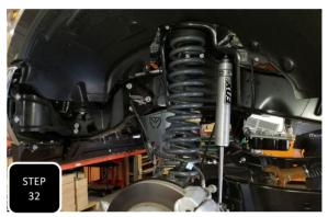
**Step 32** Move your adjustable jack under the driver's side of the axle and apply pressure so that you can remove the lower shock bolt and then lower the axle down. Next, Install the new lift coil with the factory rubber isolator on top, jack the axle back up and re-attach the shock. Repeat this step on the other side.
