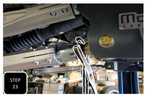
**Step 23** Tighten down all 4 of the M8 pinch bolts and then cinch down the two jam nuts on the rod ends. Repeat steps 15-23 on the other side.
