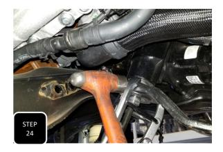
**Step 24** Using a 46mm socket, remove the pitman arm mounting nut. Next, apply tension to the arm using a pitman arm puller or a suitable 3 jaw puller. Hit the side of the pitman arm, right at the steering shaft, with a hammer a few times, very hard and then tighten down the puller some more. Proceed doing this until the pitman arm separates from the steering box. **NOTE: BE CAREFUL NOT TO DAMAGE THE STEERING BOX OR STEERING SHAFT.**
