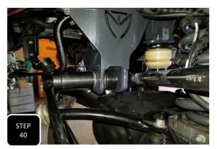
**Step 40** When attaching the trac bar to the drop down bracket, you will need to use the provided off-set plates. The hole will need to be off-set to the driver's side for the 4" lift or towards the passenger side for the 8" lift. Use the factory M18 bolt and nut and only loosely attach for now. **NOTE: THE TRAC BAR WILL GET FULLY TIGHTENED WHEN THE TRUCK IS ON THE GROUND AT RIDE HEIGHT.**
