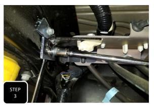
**Step 3** Unbolt the rear brake line guide bracket on the inside of the driver's side frame rail and install the provided drop down bracket using one of the factory bolts at the frame and the provided M8 bolt, nut, and washers at the bracket.
