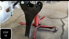
**Step 16** Loosen all 3 radius arm mounting bolts, 2 at the axle and 1 at the frame and then remove the radius arm. **NOTE: WORK ON ONE SIDE AT A TIME SO THAT THE AXLE IS SAFELY SUPPORTED AT ALL TIMES.**
