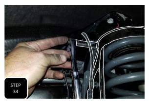
**Step 34** Separate both ABS line guide clips from the front of the coil bucket on the frame and install the new ABS/brake line bracket using the provided M8 bolts, nuts, and washers. **NOTE: THE DRIVER'S SIDE BRACKET IS THE LONGER OF THE TWO PROVIDED BRACKETS.**
