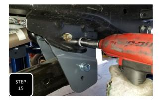
**Step 15** Repeat steps 11-14 on the passenger's side and then tighten the bolts attaching the bracket to the frame, the M18 bolt gets torqued to 200 ft/lbs, the 3/8" to 50 ft/lbs and the M12 socket head bolt to 50 ft/lbs. The radius arm bolts will not get tightened until the truck is on the ground at ride height.
