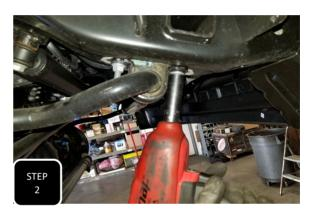
Step 2 Unbolt the sway bar from both end links and the frame on both sides and remove.
