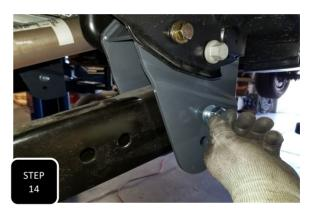
**Step 14** Swing the radius arm up and attach it to the lower hole of the new bracket using the provided M18 bolt, nut, & washers. For a 4" lift attach the arm to the upper of the two holes and for a 6" or 8" lift attach it to the lower of the two holes.
