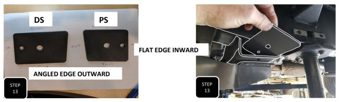
**Step 13** Locate the flat plate labeled DS and slide it into the cross member above the back of the radius arm bracket. Line up the hole and loosely attach the plate and bracket together using the provided M12-1.5 X 40 socket head allen bolt. **NOTE: THE DRIVER'S SIDE IS THE LONGER OF THE TWO PLATES.**
