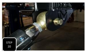
**Step 20** Locate the other arm that matches the one you just installed, adjust it to an eye-eye length of 32" and grease the rod end. Next, loosely install it into the bottom hole of the 4 link frame bracket using the provided 9/16" bolt, washers, and nut. **NOTE: THE ROD ENDS ARE NOT PRE-GREASED AND REQUIRE GREASE FOR PROPER FUNCTION.**
