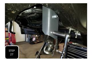
**Step 27** Using the provided M10 bolts and washers, attach the new steering stabilizer drop down bracket to the inside of the passenger side frame with the welded shim touching the frame and tighten. Next, attach the factory bracket to the lower half of the drop down bracket using the other provided M10 bolts, nuts, and washers. **NOTE: THE FACTORY BRACKET WILL MOUNT INSIDE OF THE PROVIDED BRACKET.**
