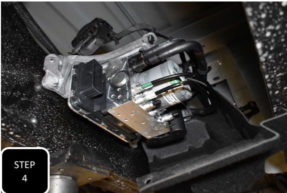
Step 4 Locate the air ride valve block on the passenger side frame rail and crack open the two lines leading to the rear air bags to bleed the air out of them. Once the bags have been deflated, tighten up both fittings.
