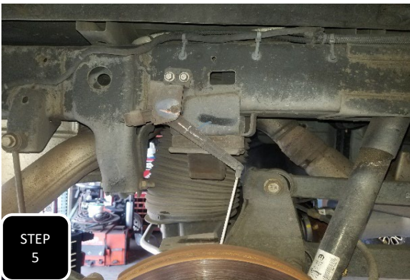
Step 5 Disconnect the sensor rods from the axle using a suitable pry tool. The plastic rod end will pop off of the metal mounting ball with a good amount of pry force.
