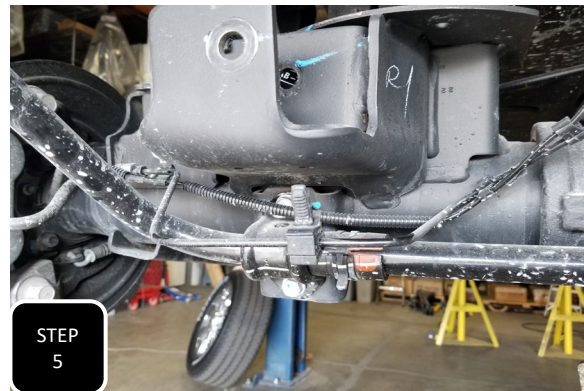
Step 5 Disengage the guide clip attaching the brake line to the bottom of the trac bar bracket and pull down a bit so it is out of the way.
