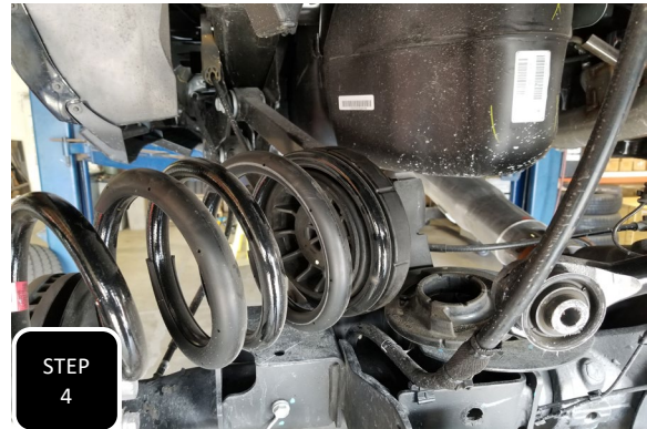
Step 4 Unbolt the sway bar end links from the frame on both sides and spin them out of the way. Next, lower the axle and remove both of the rear coils.
