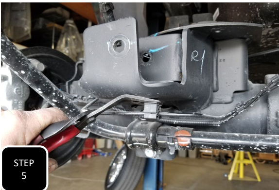
Step 5 Disengage the guide clip attaching the brake line to the bottom of the trac bar bracket and pull down a bit so it is out of the way.
